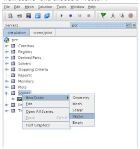
4. In the newly created vector scene, expand "Displayers" followed by "Outline 1" and click on "parts". From the properites menu of parts, select only the "plane section" that was just created from the list. Next under "vector 1" in the parts menu, select only "plane section" again. The vector field is the velocity field by default.
