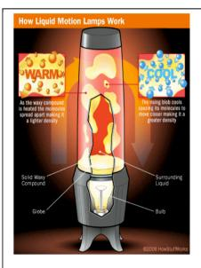
Figure 1: Convective flow in a lava lamp
