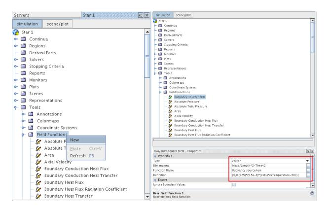
7. Now under "fluid\_medium" in "Regions" tab, change the "Momentum Source Option" from "none" to "specified". Now under the "Physical Values" tab change the method of the "Momentum Source" to "Field Function" from the default "Constant". Select "Buoyancy source term" from the list of available field functions.
