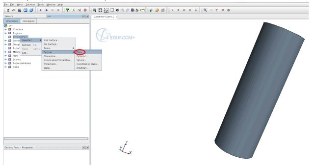
2. For the "input parts" choose the "fluid\_medium" parameter and make sure the "normal" to the x component is 1. click on "create".
