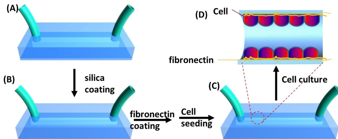
**Figure SI2.** Fabrication of a microfluidic device and cell culture in the device.
