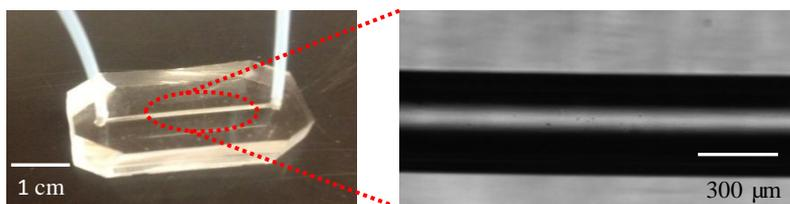
**Figure S11.** A photograph of a microfluidic device with microchannels coated with a layer of glass and optical microscopic image of the glass coated microchannel.
