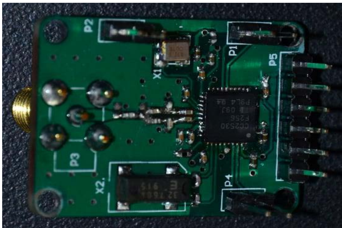
Fig. S1 Photograph of the print circuit board (PCB) of wireless communication module based on the chip CC2530. The CC2530 is a true System-on-Chip (SoC) solution for IEEE 802.15.4, Zigbee applications. It enables robust network nodes to be built with very low total bill-of-material costs. The CC2530 combines the excellent performance of a leading RF transceiver with an industry-standard enhanced 8051 MCU, in-system programmable flash memory, 8-KB RAM, and many other powerful features. The CC2530 comes in four different flash versions: CC2530F32/64/128/256, with 32/64/128/256 KB of flash memory, respectively. The CC2530 has various operating modes, making it highly suitable for systems where ultralow power consumption is required. Short transition times between operating modes further ensure low energy consumption.
