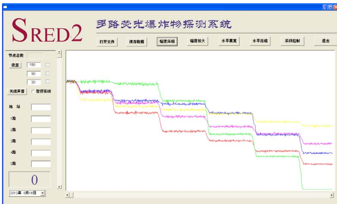
Fig. S3 The complete interface of the control panel, where the five curves stand for the test results of five sensor channels. The seven steps in the curves correspond to the test results from samples of different concentrations: 0, 10, 20, 30, 40, 50, 60 \mu\text{M} .
