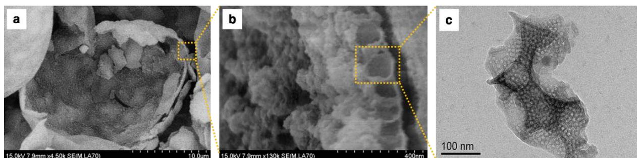
**Fig. S5** SEM (a, b) and HR-TEM (c) images of a fractured silica particle (HMS-3) showing the hierarchical trimodal (i.e., giant, macro, and meso) porous structure.
