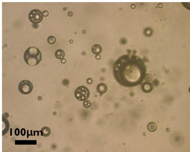
**Fig. S2** Optical micrograph image of double emulsion droplets prepared under a high-shear mixing. Both internal and external droplets have highly polydisperse size distributions.
