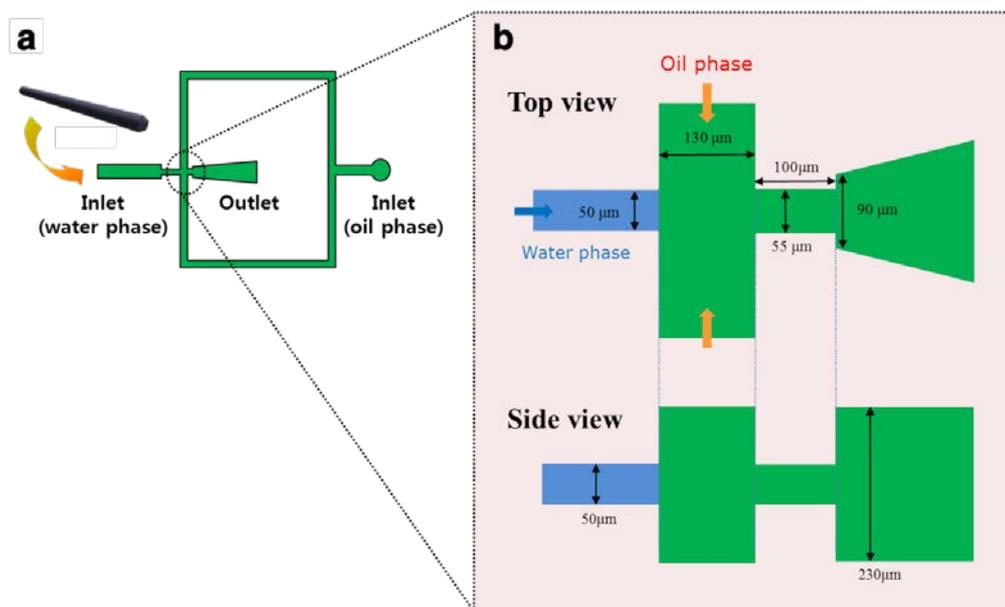
**Fig. S1** Schematic diagram of a 3-D microfluidic flow-focusing device. (a) Overview of the device. The glass capillary was inserted into the dispersed (water) phase channel, which is open on one end. (b) Top and side views of the orifice region enclosed by the circle in (a).
