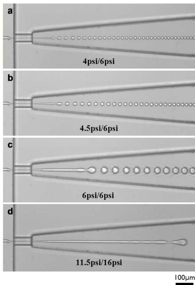
**Fig. S3** Representative still images of the droplet breakup process at the indicated pressure ratios ( $P_w/P_o$ ). Double emulsions and triple emulsions with a single internal droplet were obtained from (a, b) and (c), respectively. (d) The elongated jet produced double emulsions with multiple internal droplets, as shown in Fig. 3d.
