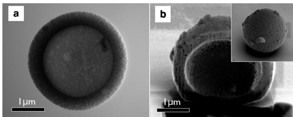
**Fig. S4** STEM (a) and SEM (b) images of silica particles (HMS-2) prepared with 0.93% mass concentration of F127 surfactant in water (%w/v). The insets of b shows the surface topography of particles before focused ion beam (FIB) milling.
