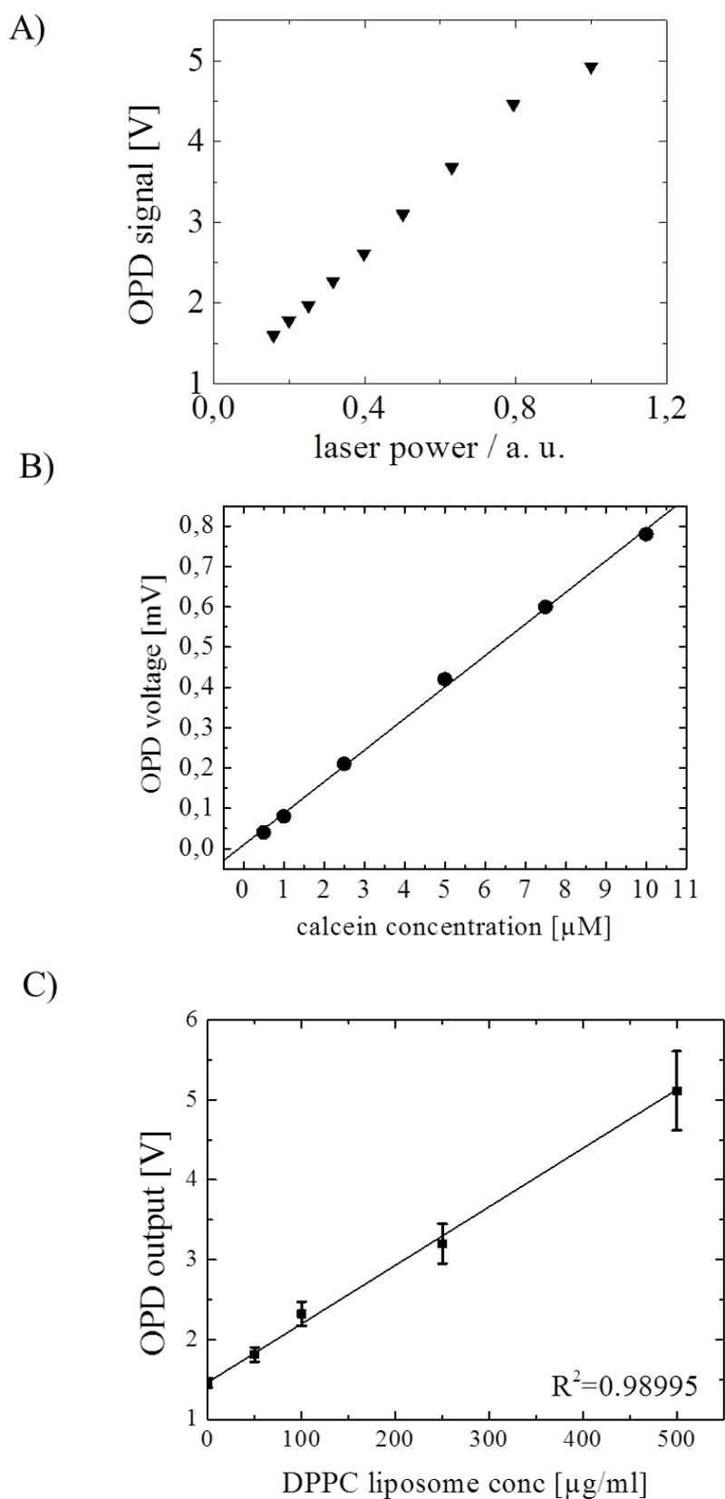
**Suppl. Fig. 2:** A) OPD voltage output in the presence of increasing laser power. B) OPD array (design#1 of Fig.1b) signals for increasing concentrations of the fluorescence dye Calcein (0.5 – 10 $\mu\text{M}$ ). C) Light scattering signals of increasing concentrations of liposomes (DPPC 200nm dia.)
