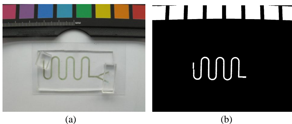
Figure S2. Picture of a captured image (a) during the experimental procedure showing the colour reference chart/patches and flow channel. Mask image (b) after image processing algorithms are applied.
