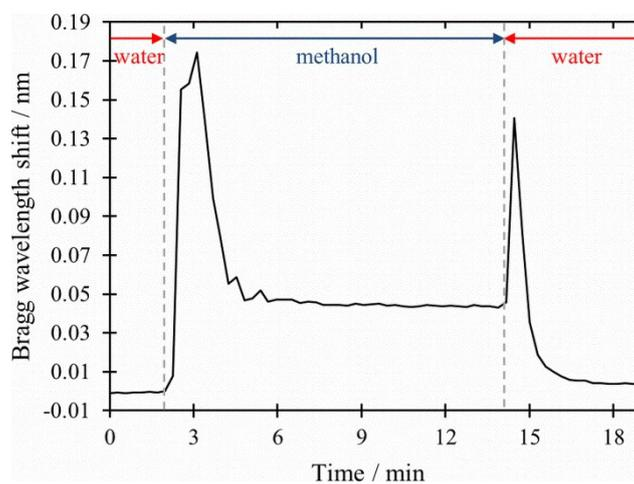
**Fig. S6** The change in Bragg wavelength upon cycling between methanol and water using a peristaltic pump.
