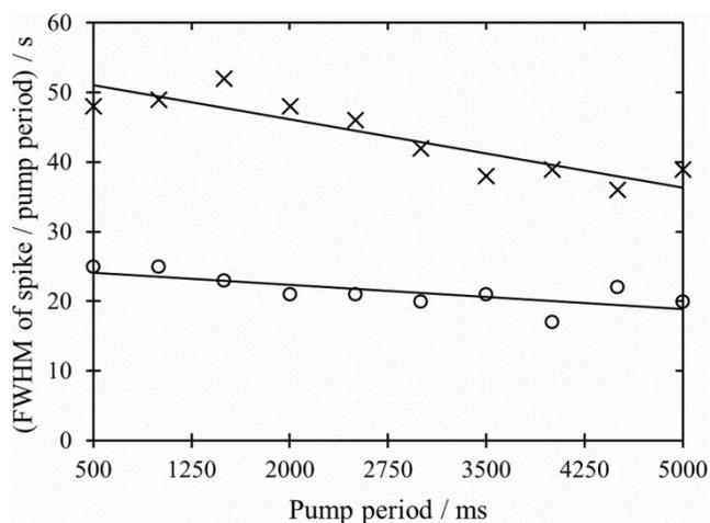
**Fig. S5** Comparison of a range of transitions as a function of pump cycle indicates that the period of pumping has little effect on the spike duration, for both the water-methanol (x) and methanol-water (o) transitions.
