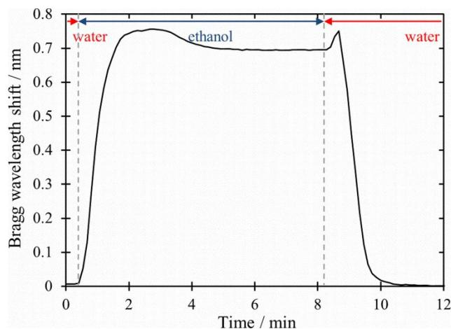
**Fig. S7** The change in Bragg wavelength upon cycling between water and ethanol, illustrating the spikes produced at the solvent interface.
