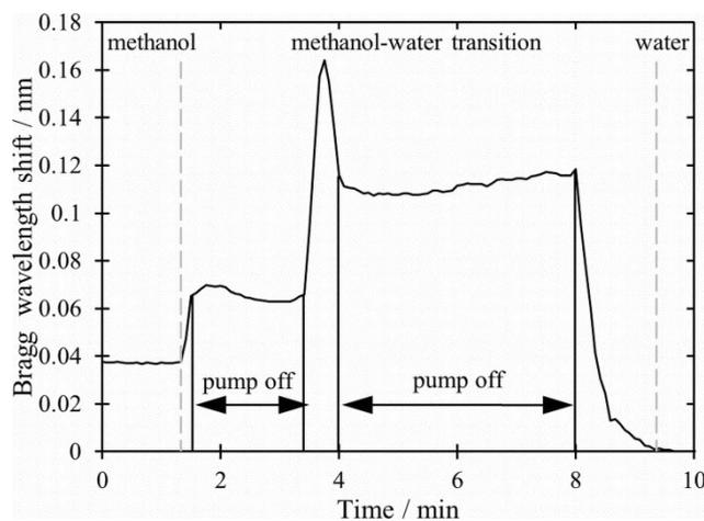
**Fig. S4** The transition from methanol to water can be paused by switching off the pump and subsequently resumed to complete the spike.
