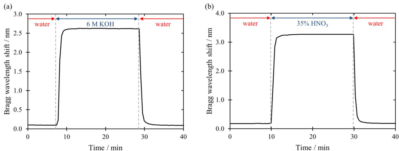
**Fig. S3** The Bragg wavelength response to cycling between water and either (a) 6.0 M potassium hydroxide or (b) 35% nitric acid, within the microfluidic system demonstrating compatibility with strong acids and bases. In both instances the transition from receding to proceeding solvent took several minutes.
