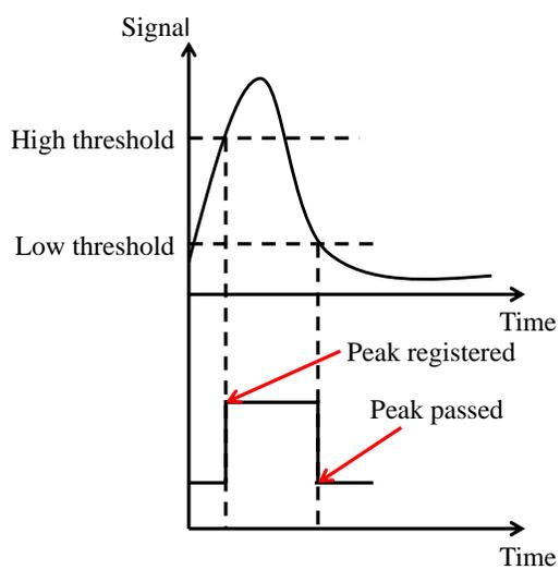
Figure S2. Illustration of a Schmidt trigger.
