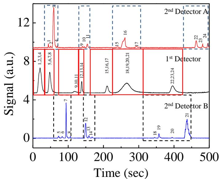
Figure S4. An enlarged part of Fig. 4(A). Solid (dashed) boxes represent the separation duration at the 1<sup>st</sup> (2<sup>nd</sup>) column, while spaces outside the solid (dashed) boxes represent the duration when the separation at the 1<sup>st</sup> (2<sup>nd</sup>) column was suspended. Note that for better illustration, the entire real-time chromatograms for 1<sup>st</sup> Detector and 2<sup>nd</sup> Detector A are vertically rearranged in comparison with the original Fig. 4(A).
