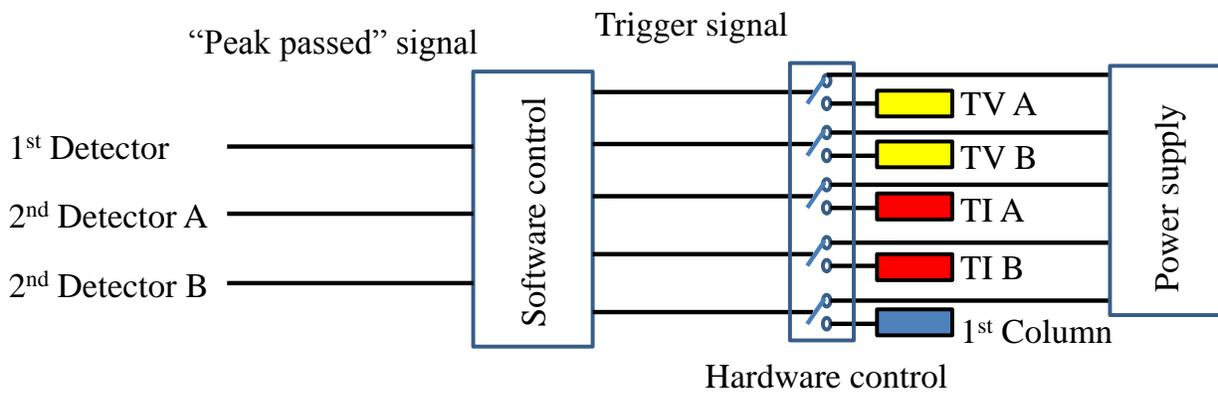
Figure S3. Schematic of the control/operation algorithm. TV: three-port valve; TI: thermal injector.
