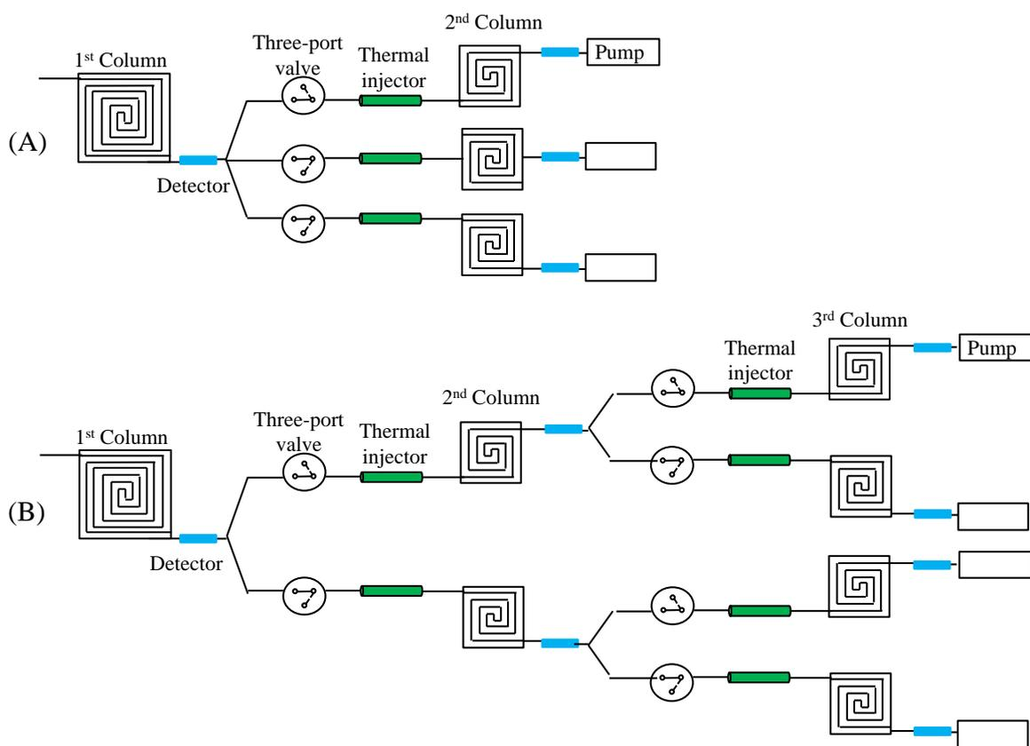
Figure S1. Conceptual illustration of (A) 1x3 channel 2-D  $\mu$ GC and (B) 1x2x4 channel 3-D  $\mu$ GC.
