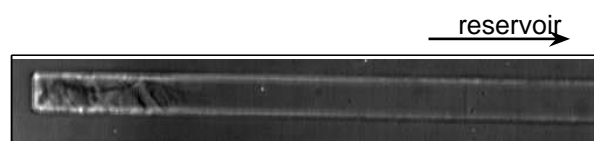
Fig. 2 Movie1.avi: movie showing the tip of a microevaporator during the continuous concentration of P104 (partially crossed polarizer and analyzer). This series shows the boundary L_1/I_1 invading the microevaporator, and the subsequent nucleation and growth of the hexagonal phase H_1 at the tip of the channel. The width of the channel is 200 \mu\text{m} and the duration of the movie is approximately 2 hours.
