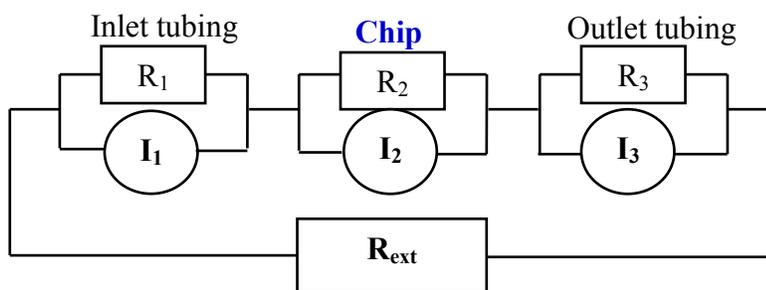
Figure 1S: An equivalent circuit of the energy conversion system
