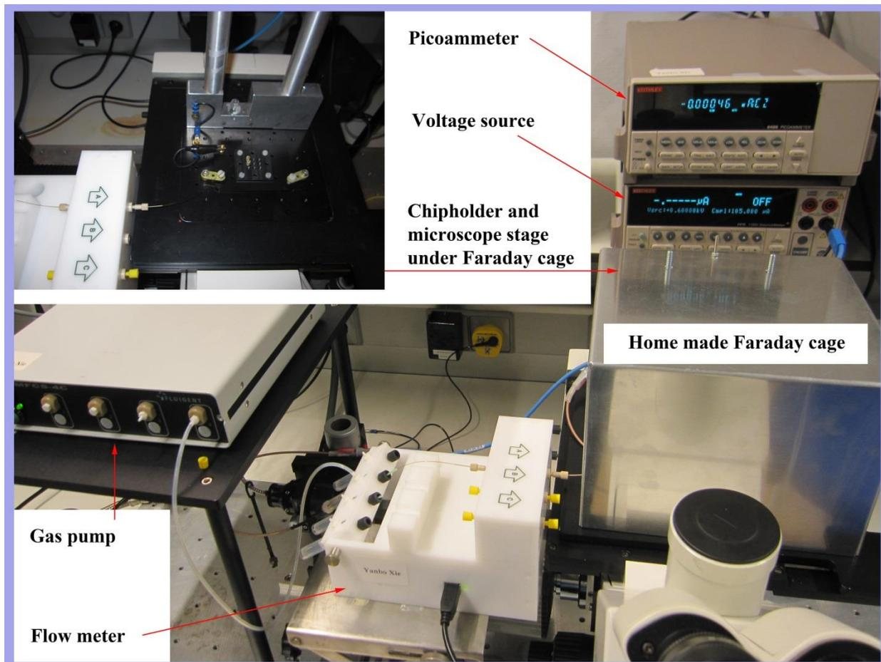
Figure 2S: Experimental setup
