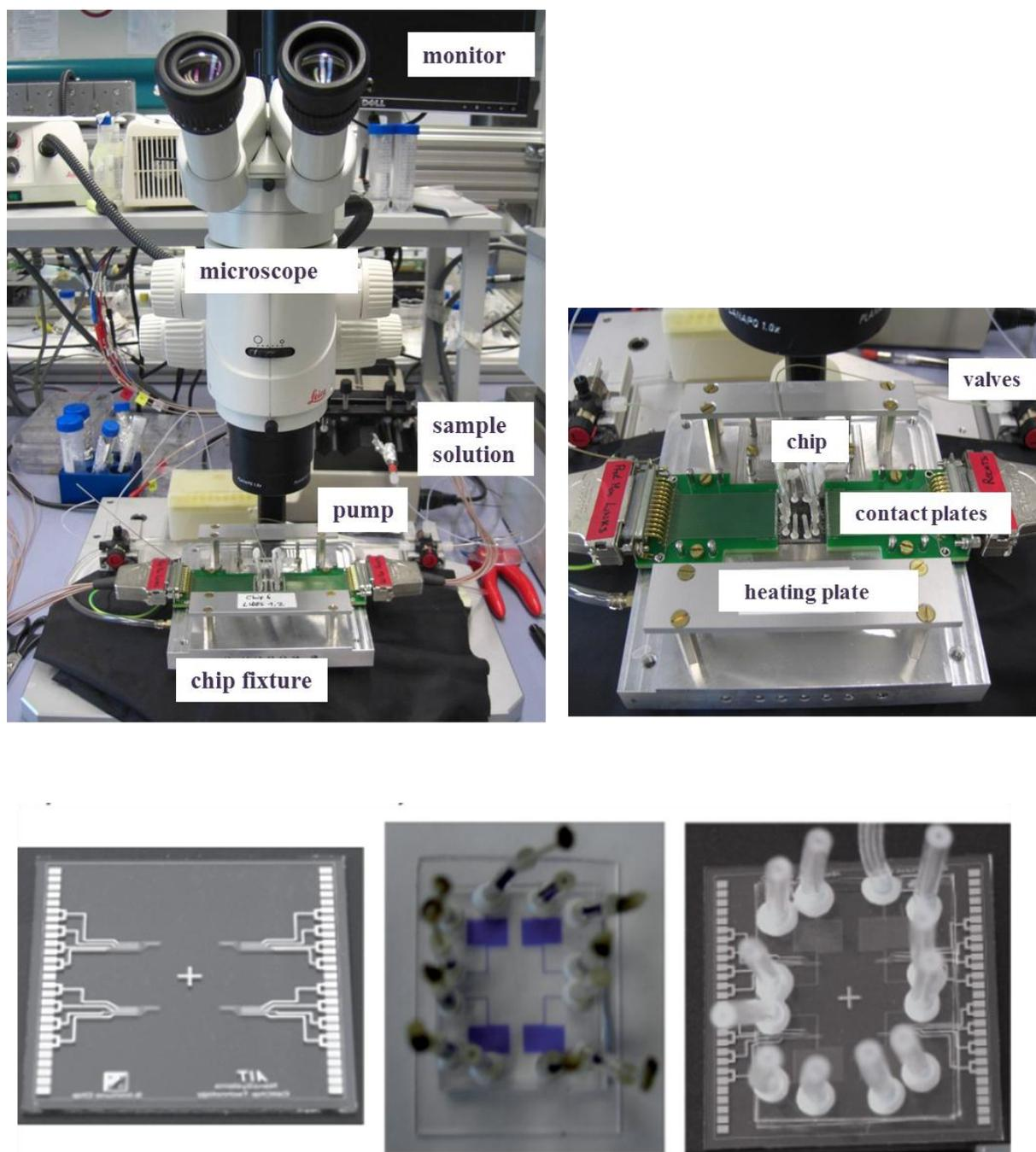
**Suppl. Fig. 1** Pictures of the LOC set up and microfluidic biochip consisting of four integrated microreactor each containing three electrode set up
