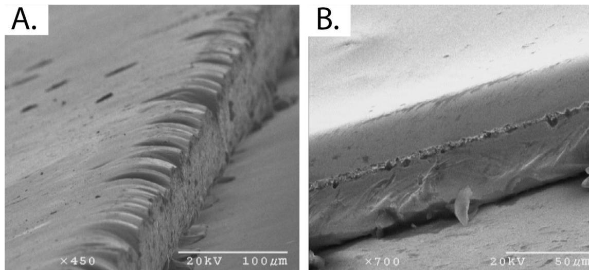
**Figure S3.** Details of nickel molds illustrating the incorporation of electroplating boundaries.
