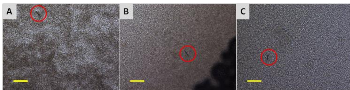
Figure S2. Motion of the rolled-up microjets in red blood cell ( \sim 5 \times 10^6 cell/ \mu\text{L} ) and serum mixture of concentration corresponding to the concentration in the blood. (A) 3% (B) 6% and (C) 9% (wt) \text{H}_2\text{O}_2 as fuel and 1% SDS. Scale bars indicate 100 \mu\text{m} .
