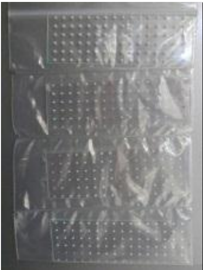
Fig.s6 Vacuum packaging of microsp sponge chips for long term storage and shipment. Four microsp sponge chips were packaged in a vacuumed plastic bag by thermal-sealing.
