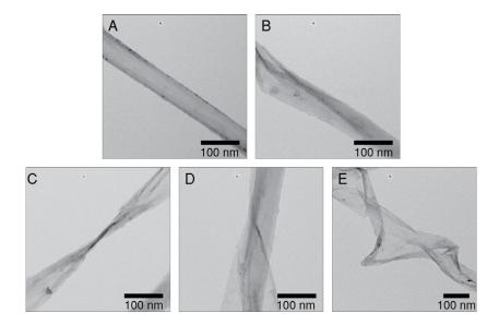
**Figure S1. Graphene Structures.** In addition to dominant nanochannel structures shown in (A) we also observe formation of different folding geometries shown in (B-E).
