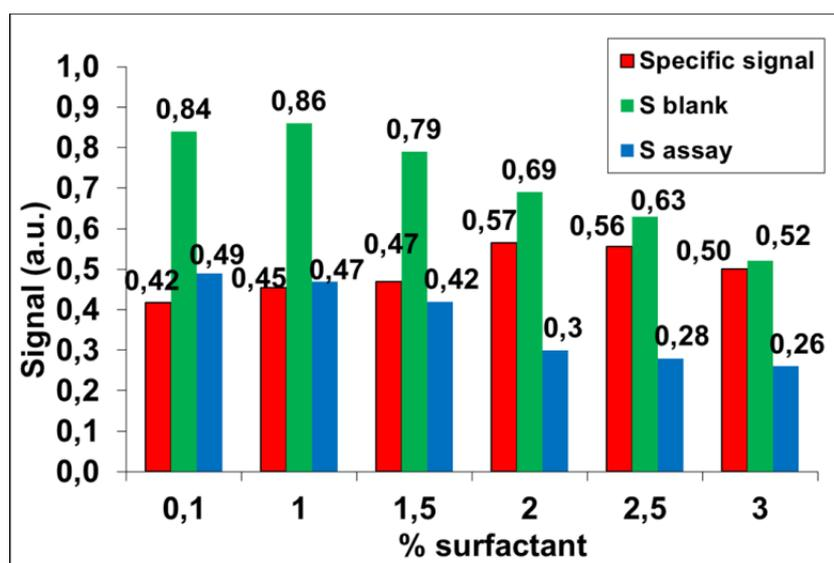
Figure S2. Influence of the surfactant percentage on  $S_{\text{blank}}$ ,  $S_{\text{assay}}$  and the specific signal  $S$ , MBs and analyte concentrations were fixed at 2 mg/mL and 1000 pM, respectively.  $B$ : 20 mT; flow rate: 0.4  $\mu\text{L}/\text{min}$ .
