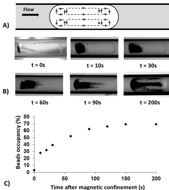
Figure S3. Schematic representation of the recirculation flows in a moving droplet. Two internal flows in the center of the droplet are surrounded by two co-rotating flows at the front and rear cap of the droplet (A). Micrographs of magnetic beads occupancy in the droplet as a
