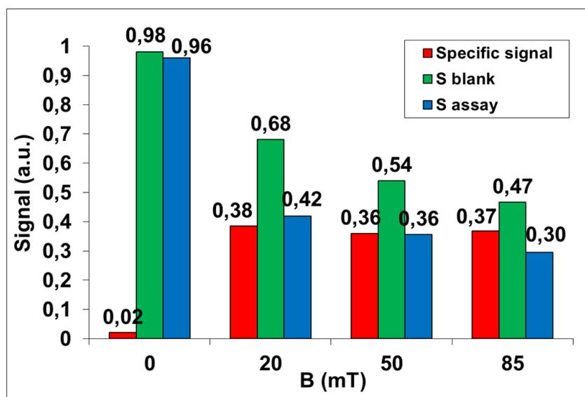
Figure S4. Influence of magnetic flux density on the specific signal,  $S_{blank}$  and  $S_{assay}$ . MB and analyte concentrations were set to 2 mg/mL and 650 pM, respectively.
