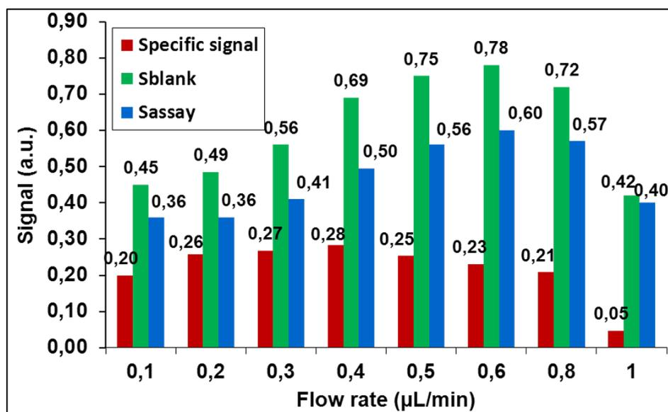
Figure S5. Influence of the flow rate on the the specific signal  $S_{blank}$  and  $S_{assay}$  for a magnetic flux density  $B = 20mT$ . MBs and analyte concentrations were set to 2 mg/mL and 650 pM, respectively.
