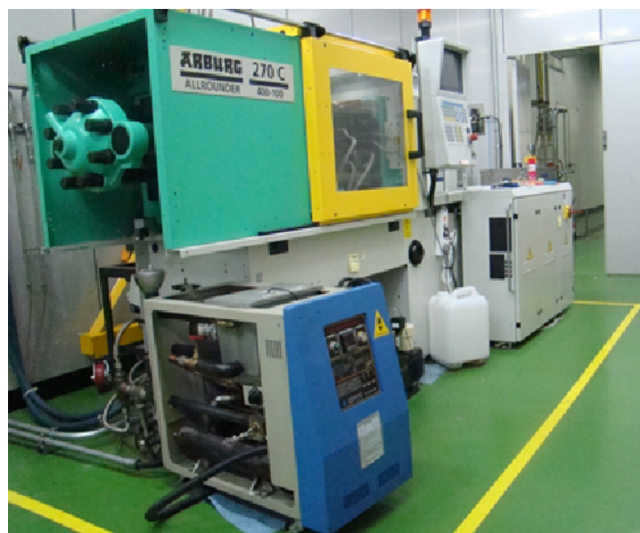
Fig. S4 The picture of the microinjection molding machine.
