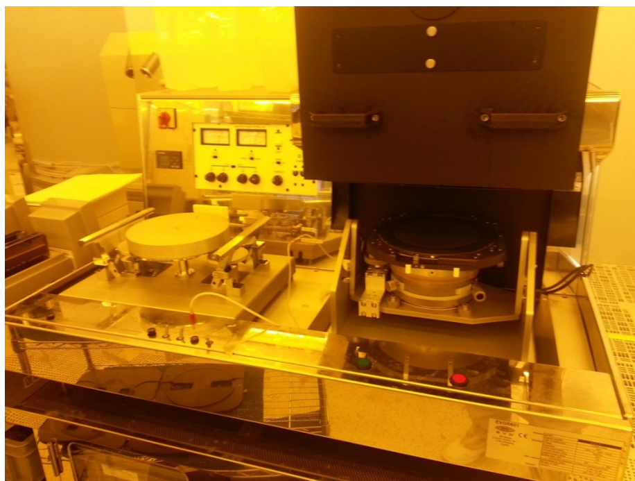
Fig. S1 The developed multidirectional tilted UV lithography system with a controllable chuck.
