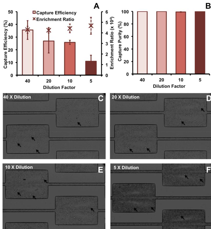
**Figure SI4.** Effect of blood dilution on capture efficiency. Performance is assessed for MCF7 cells spiked in 5X, 10X, 20X and 40X diluted blood, with around 500 cells spiked in 0.5 mL of whole blood diluted with PBS. Three independent experiments are averaged. (A) Capture Efficiency and
