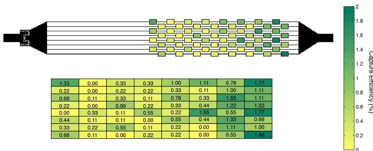
**Figure SI2.** Capture efficiency along the microfluidic chip. When 19  $\mu\text{m}$  rigid particles are injected through the device at 4 mL/min, the capture efficiency per reservoir is higher towards the end of the device. The table indicates the averaged capture efficiency in each reservoir, related to the total number of particles injected. (N=3, 300 particles injected, total capture efficiency of 35.3% for the device).
