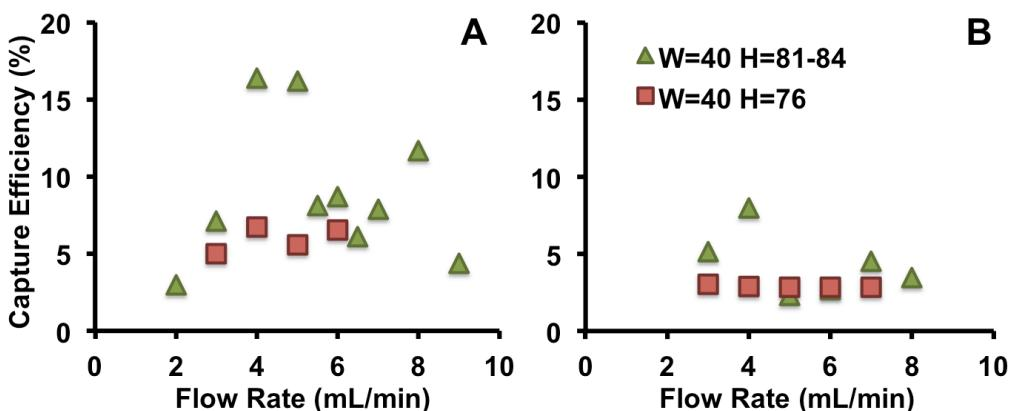
**Figure SI3.** Experimental comparison of two devices for MCF7 breast cancer cells spiked in (A) PBS and (B) healthy blood. As illustrated in Figure 2, capture efficiency varies with channel aspect ratio and flow rate. As for rigid beads, taller channels (new device) provide an improvement in efficiency over devices used previously [1].
