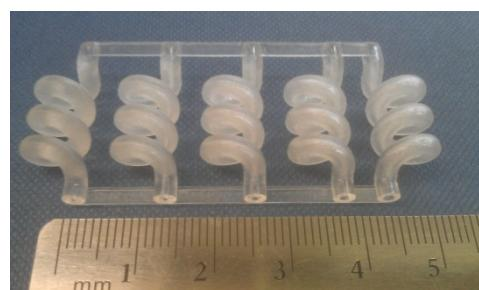
Reactor design 5 was manufactured via SL from Accura 60 resin to external dimensions of approximately 55x25x5mm. The build had a series of tubes of length 70mm, with channel diameters of 0.25, 0.375, 0.5, 0.625 and 0.75mm.
