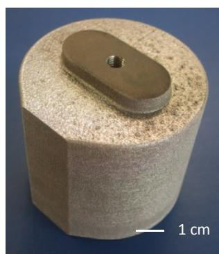
Reactor design 8 was manufactured via SLM from stainless steel to external dimensions of approximately 55x60x60mm. The reactor had a single inlet connected to an outlet by a continuous tube of length 4210 mm, diameter 3 mm and a total volume of 13.2mL.
