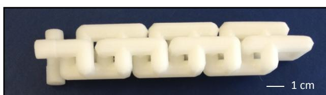
Reactor design 1 was manufactured via FDM from acrylonitrile butadiene styrene (ABS) to external dimensions of approximately 150x30x30mm. The reactor had two inlets joining at a t-piece connected to an outlet by a continuous tube of length 510 mm, diameter 3 mm and a total volume of 3.6 mL, contained within a wall thickness of 5 mm. The flow path has a split-and-recombine (SAR) mixer geometry.
