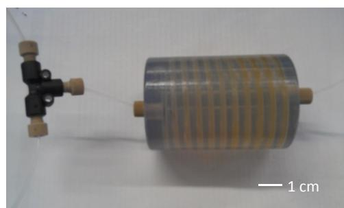
Reactor design 2 was manufactured via SL from Accura 60 resin to external dimensions of approximately 70x50x50mm. The reactor had a single inlet connected to an outlet by a continuous tube of length 3300 mm, diameter 3 mm and a total volume of 23mL.
