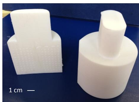
Reactor design 6 was manufactured via SLS from nylon-12 to external dimensions of approximately 70x50x50mm. The reactor had two inlets joined at an internal T-piece, connected to an outlet by a continuous tube of length 13200 mm, diameter 2 mm and a total volume of 41mL.
