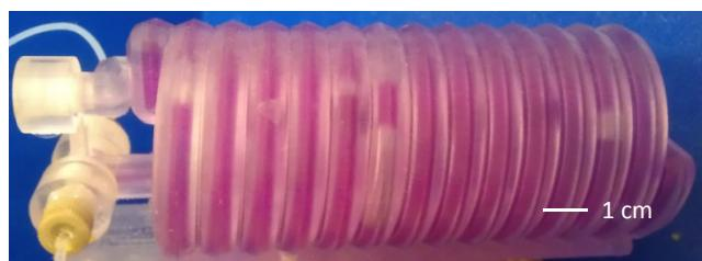
Reactor design 4 was manufactured via SL from Accura 60 resin to external dimensions of approximately 140x50x50mm. The reactor had two inlets joined at an external T-piece, connected to an outlet by a continuous tube of length 2320 mm, diameter 3 mm and a total volume of 16.4mL. The
