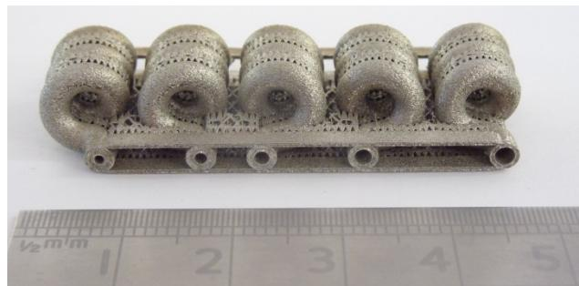
Reactor design 9 was manufactured via SLM from stainless steel to external dimensions of approximately 55x25x5mm. The build had a series of tubes of length 70mm, with channel diameters of 1, 1.25, 1.5, 1.75 and 2mm.
