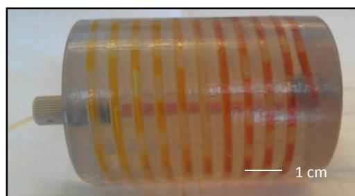
Reactor design 3 was manufactured via SL from Accura 60 resin to external dimensions of approximately 70x50x50mm. The reactor had two inlets joined at an internal t-piece, connected to an outlet by a continuous tube of length 3300 mm, diameter 3 mm and a total volume of 23mL.
