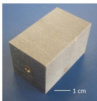
Reactor design 7 was manufactured via SLM from stainless steel to external dimensions of approximately 55x30x30mm. The reactor had a single inlet connected to an outlet by a continuous tube of length 300 mm, diameter 3 mm and a total volume of 2.1mL.
