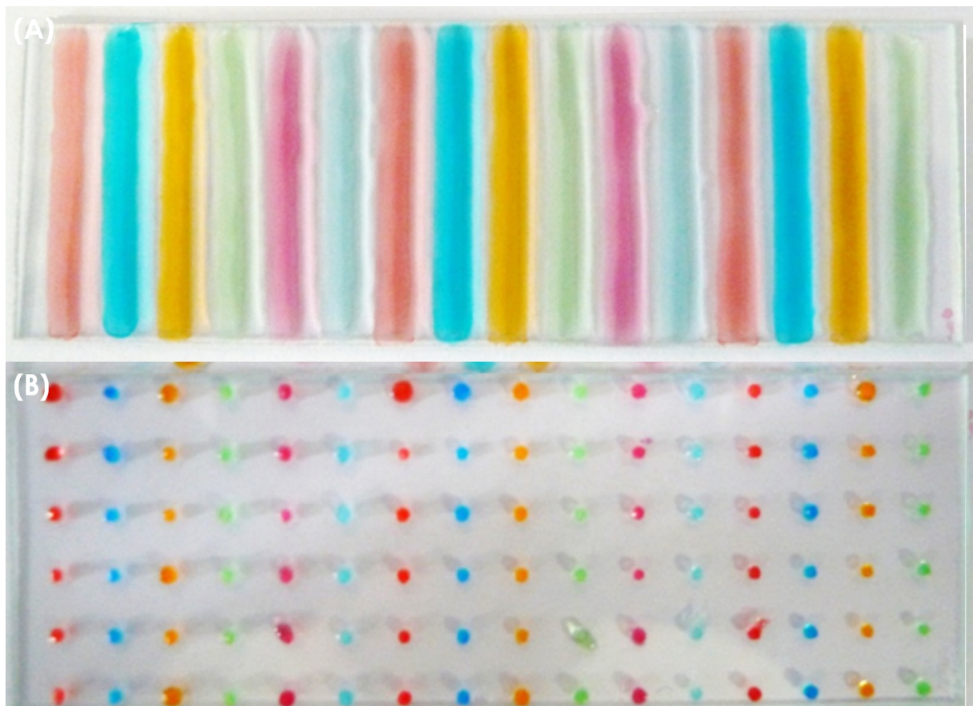
Supplementary Fig. 1 Parallel loading of food dye solution onto PEG microsponge arrays.
