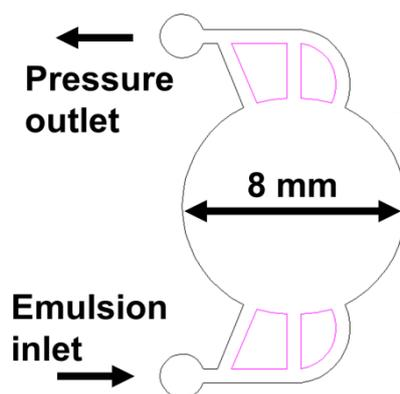
**Figure S3:** CAD-based drawing of a PDMS-based microfluidic chamber for storing water-in-oil emulsion droplets under static conditions suitable for long-term imaging.
