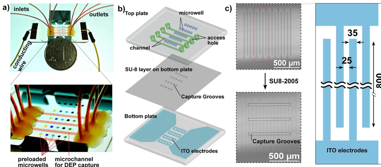
**Figure S1.** a) A photograph of the device with zoom-in view; the microchannels and microwells were loaded with dye solutions of different colors; b) Schematic illustration showed that the system was consisted of the top glass plate, bottom plate with 5  $\mu\text{m}$  SU-8 coating and ITO microelectrodes; c) Interdigitated ITO microelectrodes before and after fabricating three capture grooves. The detailed geometry was shown in the zoom-in schematic drawing.
