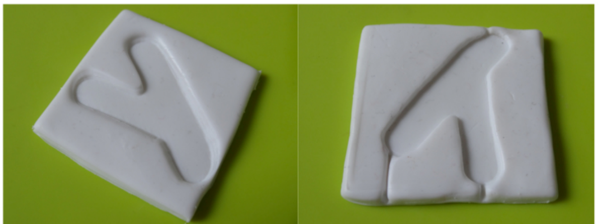
56 S3. Y-shape channel (left) without inlet/outlet and with inlet/outlets (right) made with a toothpick.
