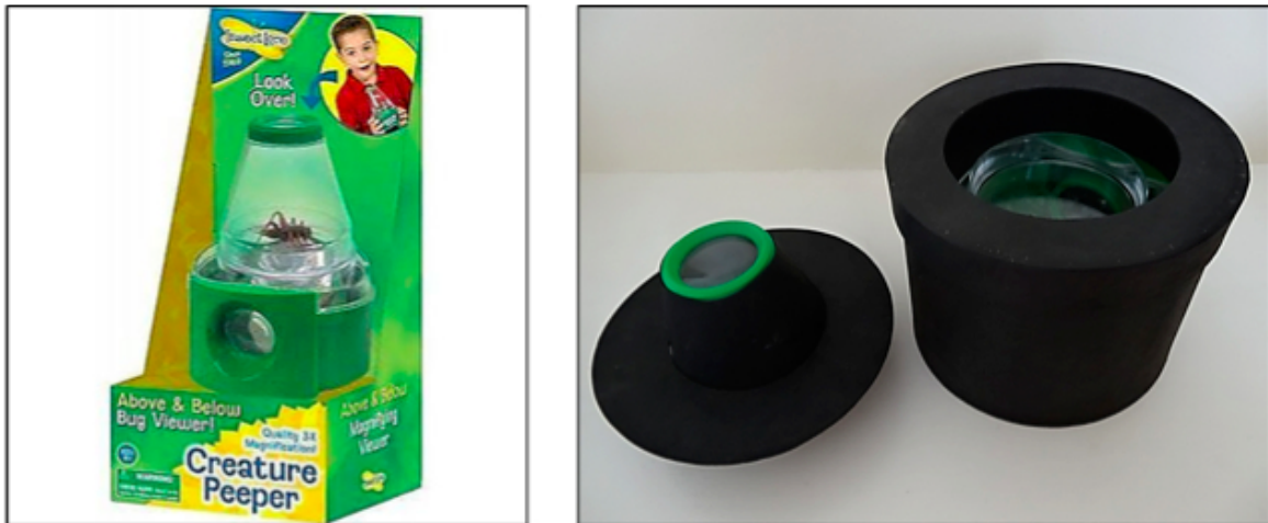
163 Figure S8. Left: Insect magnifier used for reproducing the microscope. Right: Black cardboard box 164 with the magnifier to visualize by fluorescence the magnetic beads trapped onto the bad red particles.
