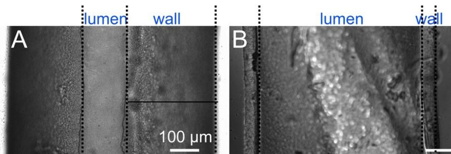
**Fig. S3** Microscopic images showing cellulose microtubes with inner diameter of ca. 150  $\mu\text{m}$  (A) and another microtube with thickness ca. 50  $\mu\text{m}$  (B).
