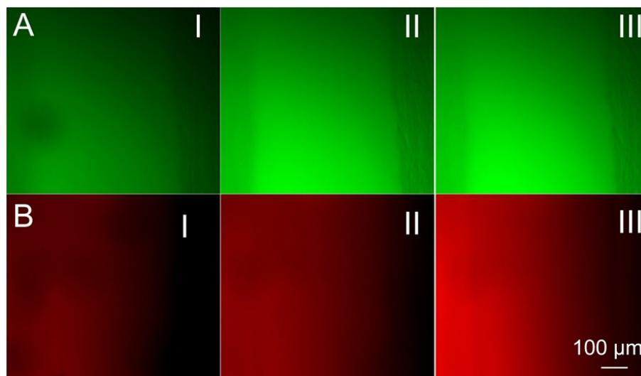
**Fig. S4** Fluorescence microscopic image showing the gradient generation of FITC-dextran ( $M_w = 20 \text{ kDa}$ ) (A) and Rhodamine-dextran ( $M_w = 70 \text{ kDa}$ ) (B) between adjacent cellulose lumens over time, The time of I, II, III is 15 min, 24 h, 48 h.
