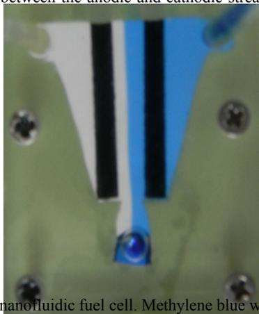
Figure S2. Top view photograph of the nanofluidic fuel cell. Methylene blue was used as colorant at  $200 \mu\text{L min}^{-1}$  flow rate
