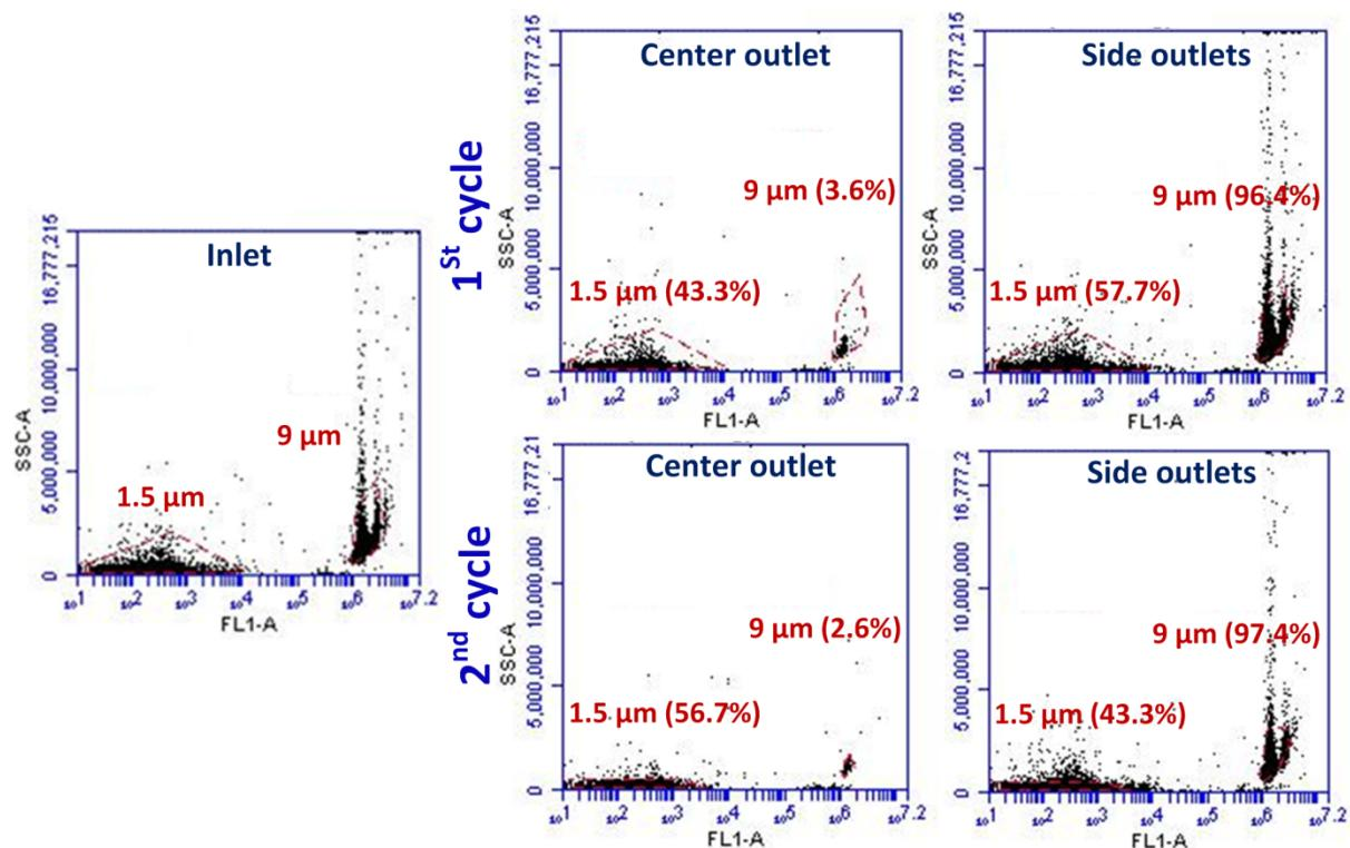
**Figure S3:** Scatter plots captured using flow cytometer (Accuri C6, BD Biosciences, USA) showing the results of separations of particle mixtures in a microfluidic device (30/90 design, 1:1:1).
