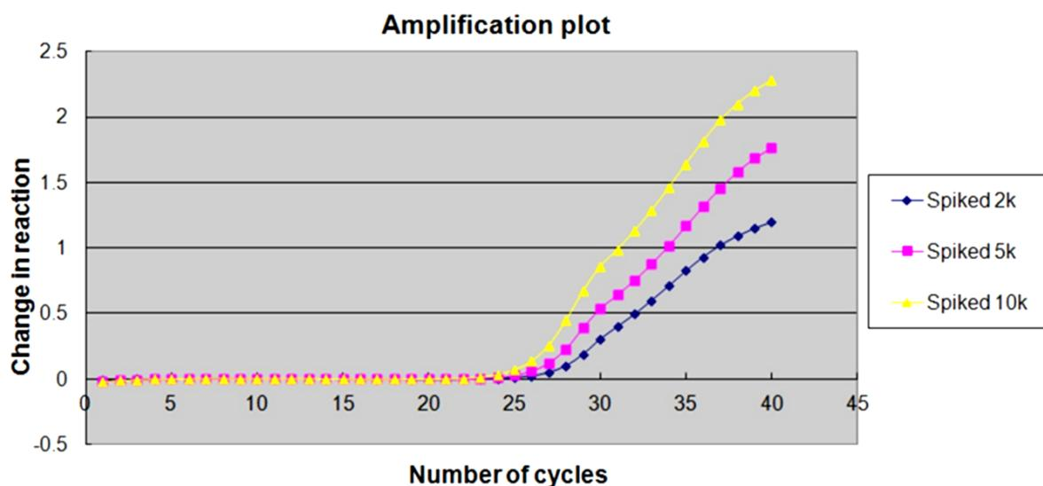
**Figure S2:** Calibration curve generated with qPCR data for estimation of parasite recovery.
