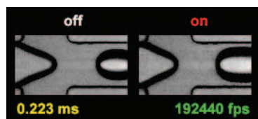
Video01.mp4 Gas-liquid interface motion at off and on mode capturing at 192440 FPS
