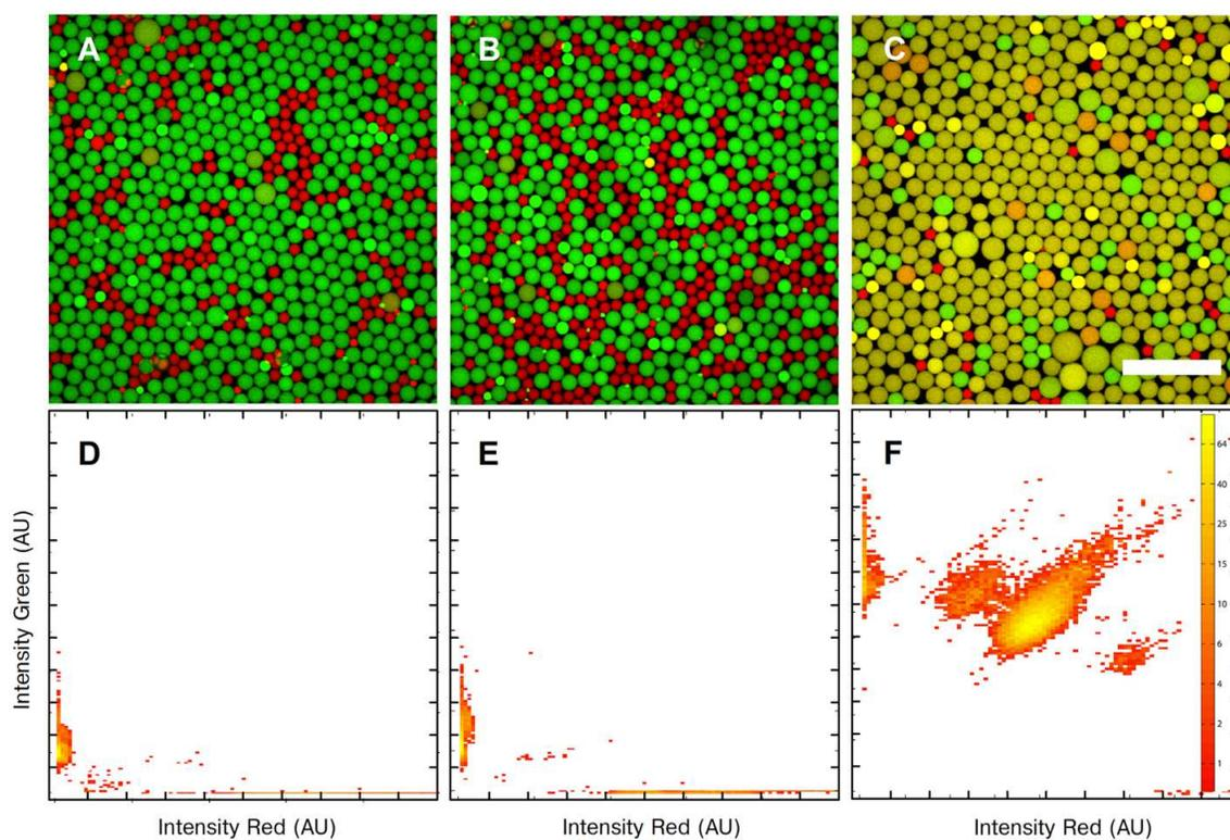
**Fig. S4** Two-color overlay fluorescence images of droplets collected from the outlet of the microfluidic device using: (A) HFE-7500, (B) PFO, and (C) PFB; scale bar is 150mm. 2-D histogram of all individual droplet fluorescence intensities obtained from coalesced droplet pairs in (D) HFE-7500, (E) PFO, (F) PFB.
