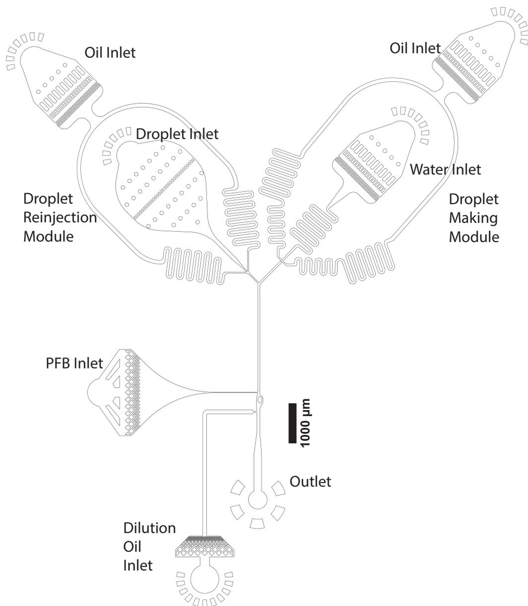
**Fig. S2** Complete scale device drawing.
