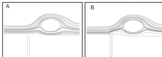
**Fig. S1** Fluid streamlines for operational flow rates in the merging microfluidic geometry generated by computation fluid dynamics in COMSOL. Flow rates for PFB addition are (A) 5  $\mu\text{L/hr}$  and (B) 100  $\mu\text{L/hr}$ .
