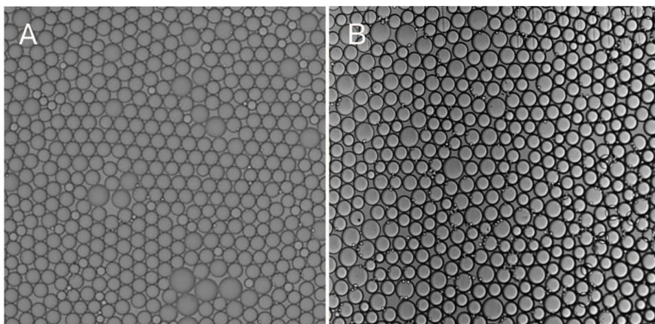
**Fig. S3** Comparison between microfluidic chemical and electro-coalescence. (A) a collected merged droplet population using PFB to destabilize, (B) collected merged droplet population using an electro-coalescence device operating at 0.8kV.
