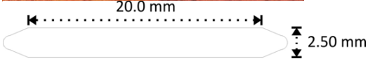
SI Figure 7. A. Image of microfluidic device for FSS studies. B. Channel geometry and dimensions.
