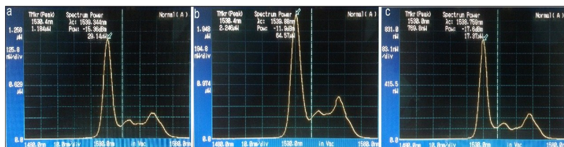
Fig. S.3. Experiment results of electro-optical modulation at 1530nm with and without a voltage applied for the ionic liquid [Emim][Nf 2 T]. a , U=0V . b , U=+3.5V . c , U=-3.5V . The input fiber and output fiber was fixed at position A and B, respectively.
