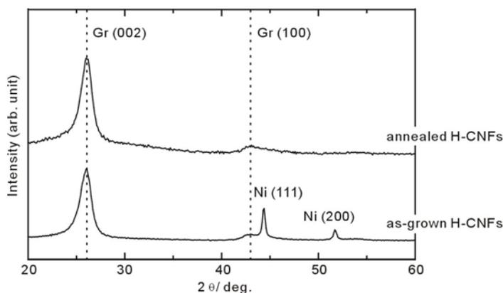
Fig. 1S XRD pattern of as-grown H-CNFs and annealed H-CNFs.
