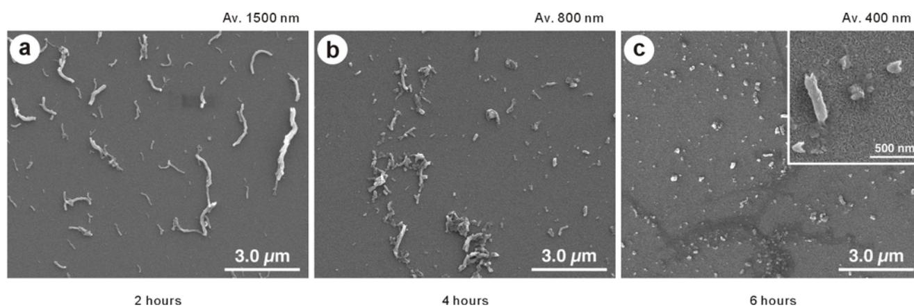
**Fig. 2S** SEM photographs of acid-sonicated H-CNFs following 2h (a), 4h (b) and 6h (c) sonication in a mixture of concentrated  $\text{H}_2\text{SO}_4$  and  $\text{HNO}_3$ . parts. This phenomenon is referred to as the “delamination effect”<sup>6</sup>, observed in layered materials such as organo-layer silicate<sup>6</sup> and graphite.<sup>5</sup>
