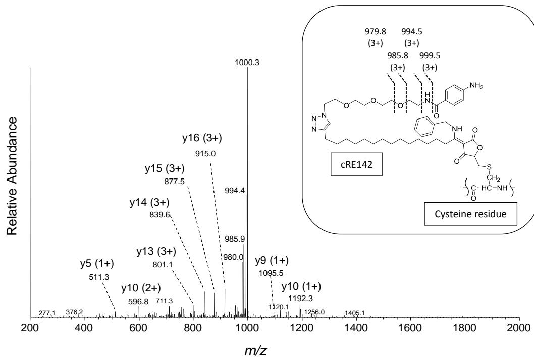
**Figure S5.** Ion-trap MS/MS (CID) spectrum of precursor ion  $m/z$  780.15. The major product ions around  $m/z$  990 appear to be derived from the fragmentation of cRE142 (insert). The insert illustrates the predicted fragmentation and the derived mass values.
