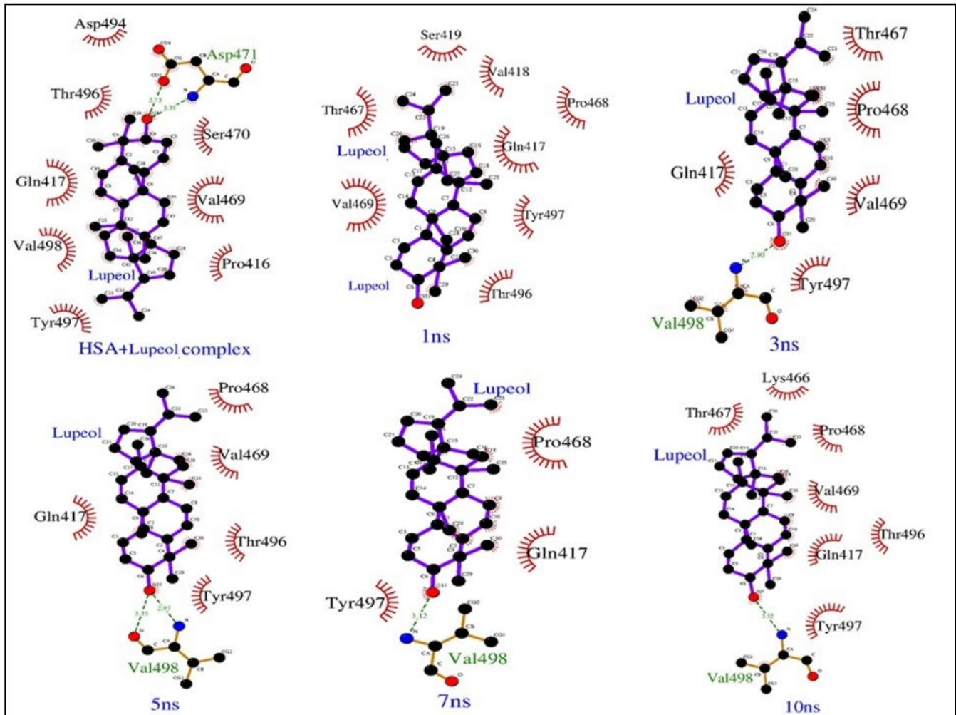
**Fig. S5** Graphical representation of the sequence of conformational changes of lupeol derivative around binding pocket. Ligplot of HSA-Lupeol derivative (Ld) showing hydrophobic interactions with subdomain IIIA at different ns (0.1 – 10 ns).
