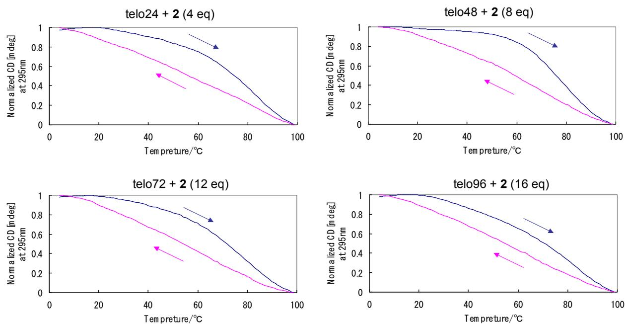
**Fig. S1** Normalized thermal melting and annealing profiles recorded at 295 nm of (TTAGGG)<sub>n</sub> (n = 4–16) in the presence of 100 mM KCl with sufficient equivalent of **2**.
