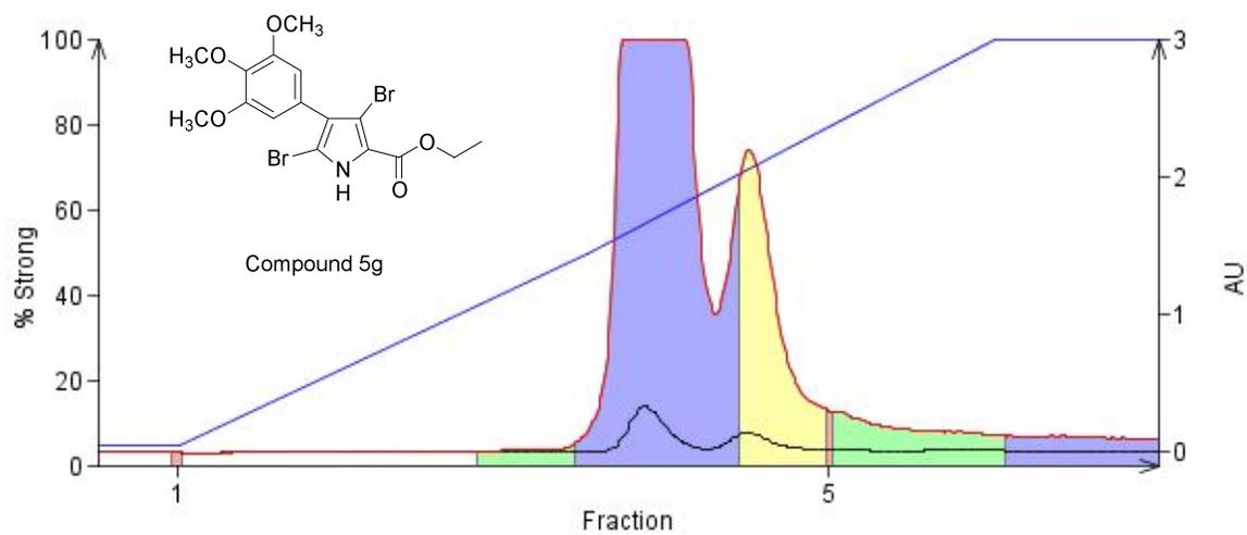
**Figure S3.** This material (**5g**) was purified on a Biotage SP-1 preparative chromatograph using a silica column with a hexane/ethyl acetate gradient. The fraction represented in blue was collected and characterized as compound **5g**.
