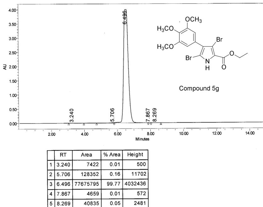
**Figure S4.** This chromatogram represents the HPLC analysis of purified compound **5g** on an Inertsil ODS-II column in an isocratic mode with a 1:1 mixture of methanol:acetonitrile.
