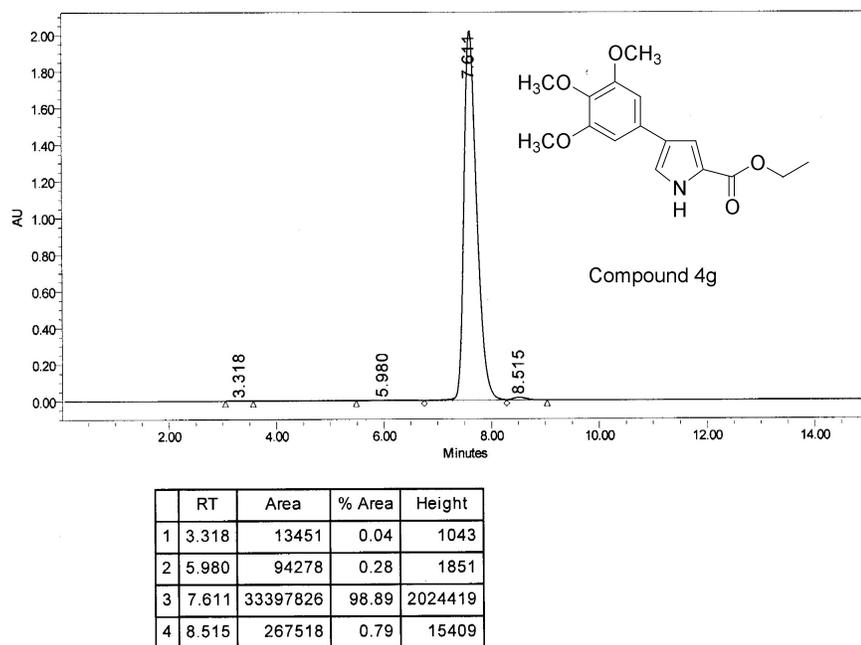
**Figure S2.** This chromatogram represents the HPLC analysis of purified compound **4g** on an Inertsil ODS-II column in an isocratic mode with a 1:1 mixture of methanol:acetonitrile.
