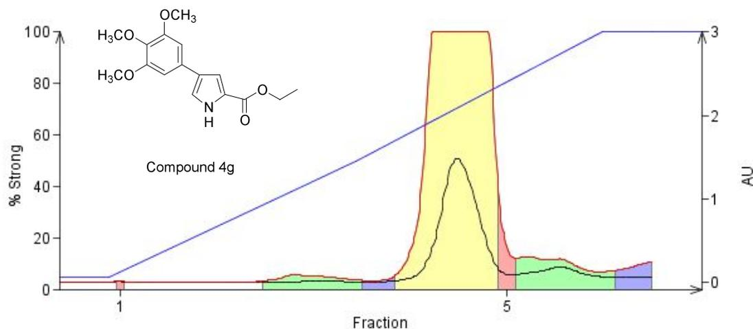
**Figure S1.** This material (**4g**) was purified on a Biotage SP-1 preparative chromatograph using a silica column with a hexane/ethyl acetate gradient. The fraction represented in yellow was collected and characterized as compound **4g**.
