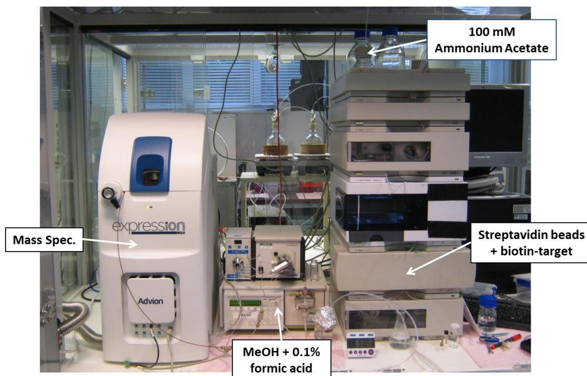
FAC assays were run on a modified Agilent 1100 HPLC system with a 100  $\mu\text{L}$  injection syringe, a 600  $\mu\text{L}$  storage loop and 100 mM ammonium acetate was used as the eluent. An Expression CMS mass spectrometer (Advion) was connected via a T-piece to the HPLC output and to a pump which delivered solution of 0.1% formic acid in methanol (make-up buffer). Stock solutions of compounds were prepared at a concentration of 50 mM in DMSO and stored at  $-20^{\circ}\text{C}$ .
