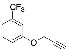
A round bottom flask, equipped with a magnetic stir bar, was charged with 3-(trifluoromethyl)phenol (0.25 mL, 2 mmol), K<sub>2</sub>CO<sub>3</sub> (1.10 g, 8 mmol), propargyl bromide (80% wt toluene, 0.89 mL, 8 mmol) and acetone (10 mL). The mixture was heated to reflux overnight and cooled to rt. The solvent was removed under pressure and water was added. The heterogeneous mixture was extracted twice
