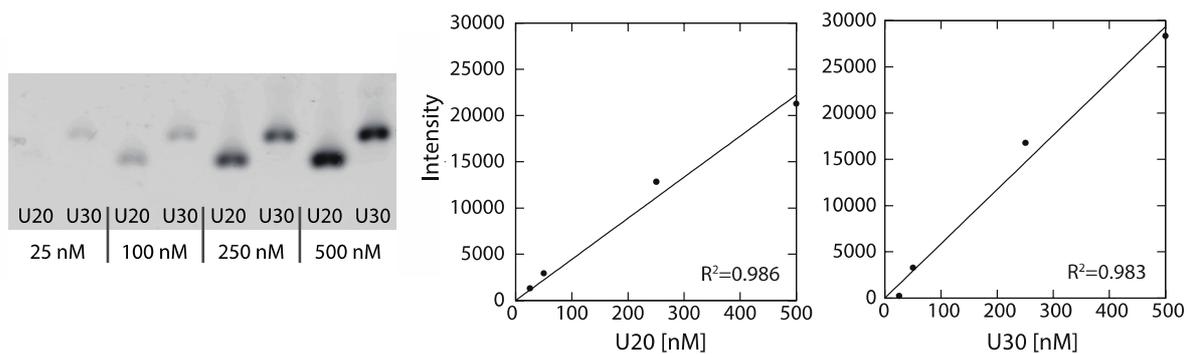
**Figure S4.** Linearity of gel-intensities and AON concentrations under HSA binding assay condition.
