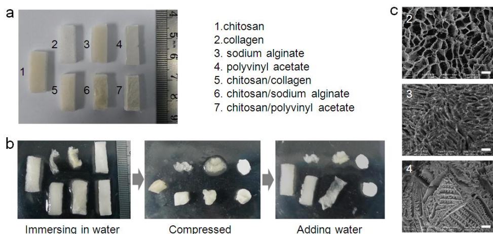
Fig. S2 Photographs and SEM images show several kinds of water soluble polymer scaffolds. (a) Photographs of several kinds of water soluble polymer scaffolds fabricated through the same freeze casting process. (b) These several scaffolds made from only one polymer are easily be dissolved in water again and show no shape-memory property except to chitosan. (c) SEM images show that different polymer scaffolds have different morphologies of microstructure. Scale bars, 100 \mu\text{m} (c).
