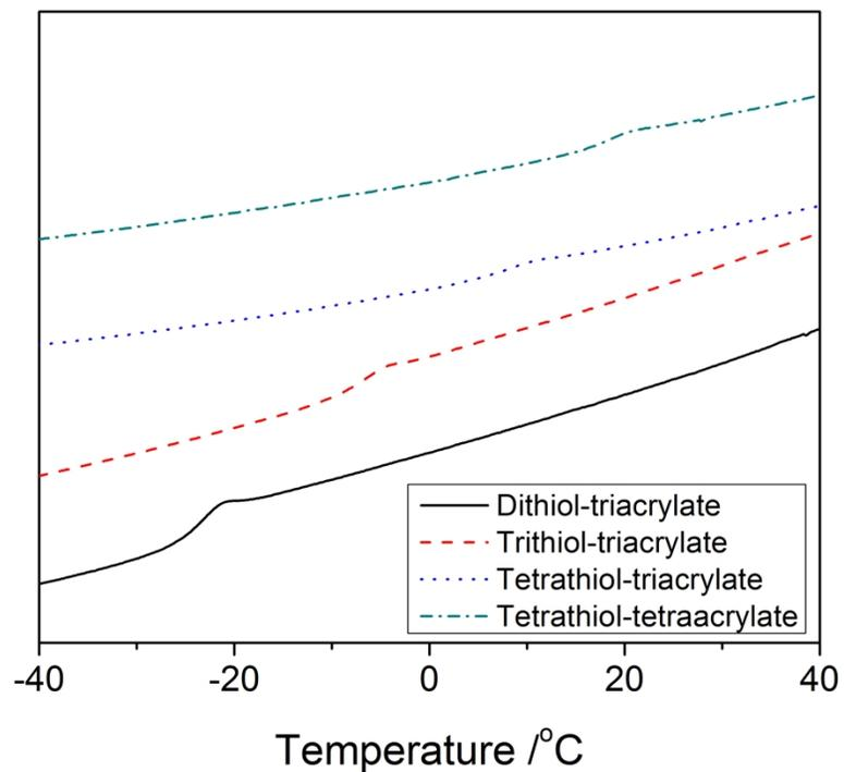
Figure S3. DSC curves of thiol-Michael microspheres made from various monomers: (a) Dithiol-triacrylate (EGBMP and TMPTA); (b) Trithiol-triacrylate (TMPTMP and TMPTA); (c) Tetrathiol-triacrylate (PETMP and TMPTA); (d) Tetrathiol-tetraacrylate (PETMP and DTPTA).
