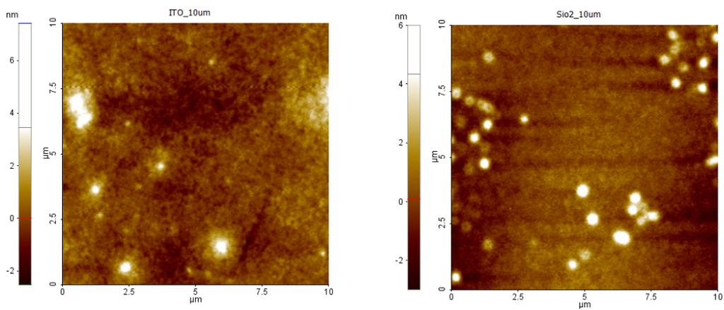
**Figure S11.** AFM image taken on a  $10\mu\text{m} * 10\mu\text{m}$  scale for DHI melanin thin films grown on (left) ITO and (right)  $\text{SiO}_2$  substrates.
