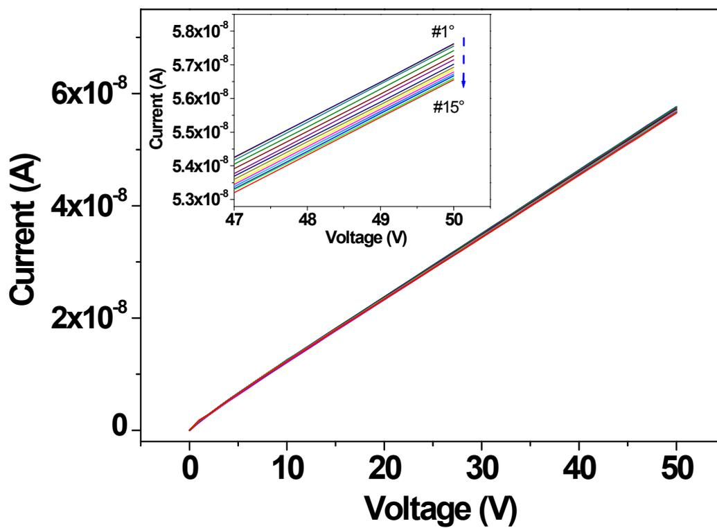
**Figure S6.** A set of repeated IV curves measured for a fresh AISSP eumelanin channel
