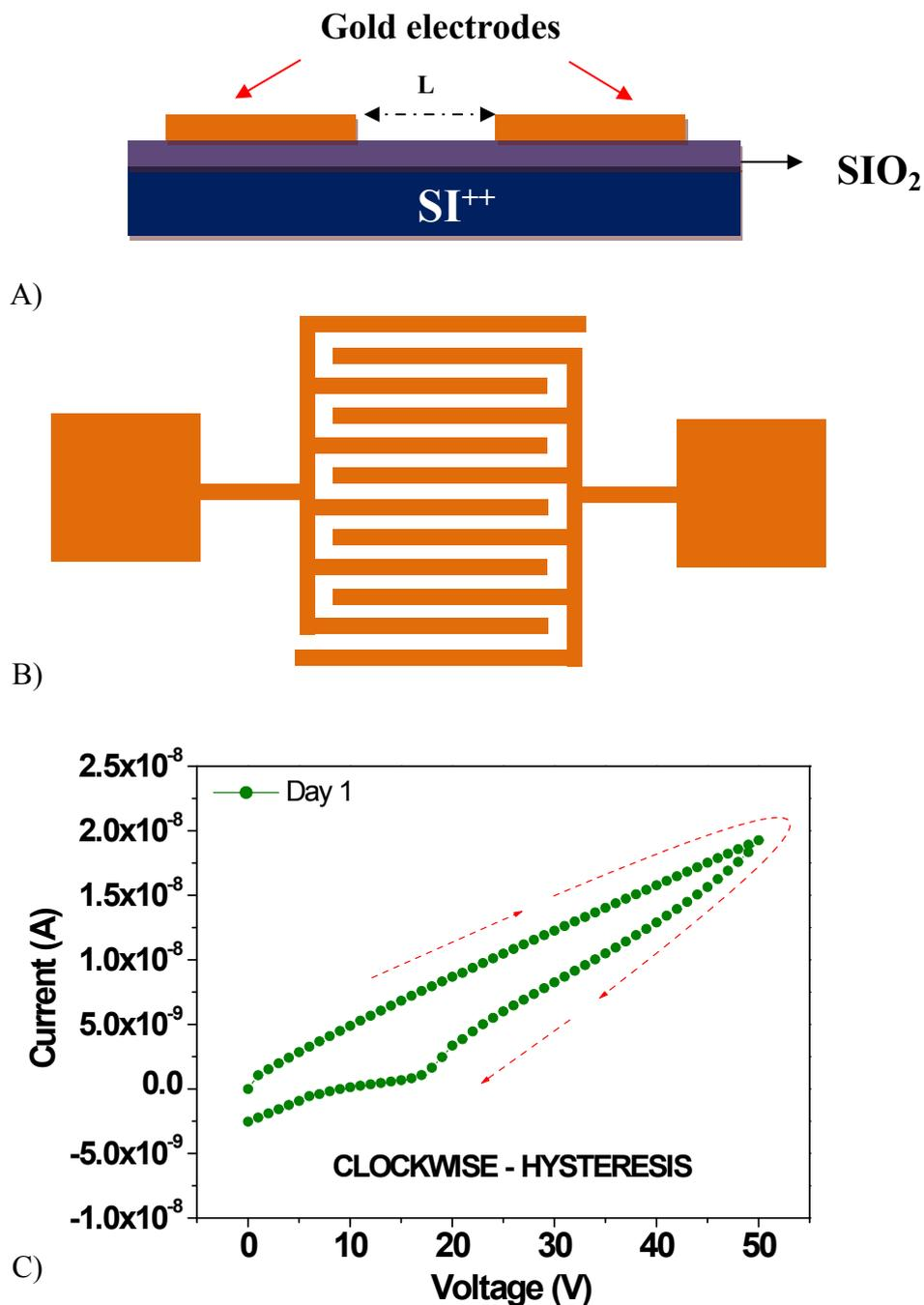
**Figure S5.** (A) Side view of the highly doped ( $\text{Si}^{++}$ )/ $\text{SiO}_2$ /Au multilayer substrates used for the electrical tests on DHI-eumelanin films. (B) Layout of the interdigitated gold electrodes. (C) Current-Voltage (IV) curve with hysteresis loop measured for a DHI melanin thin film during the first day of storage in air.
