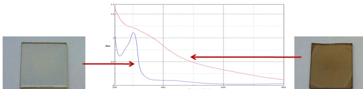
**Figure S1.** UV –vis plots of DHI and DHI melanin (120 min AISSP time) films on quartz substrates are showed with the corresponding substrate picture: DHI, left and eumelanin: right.
