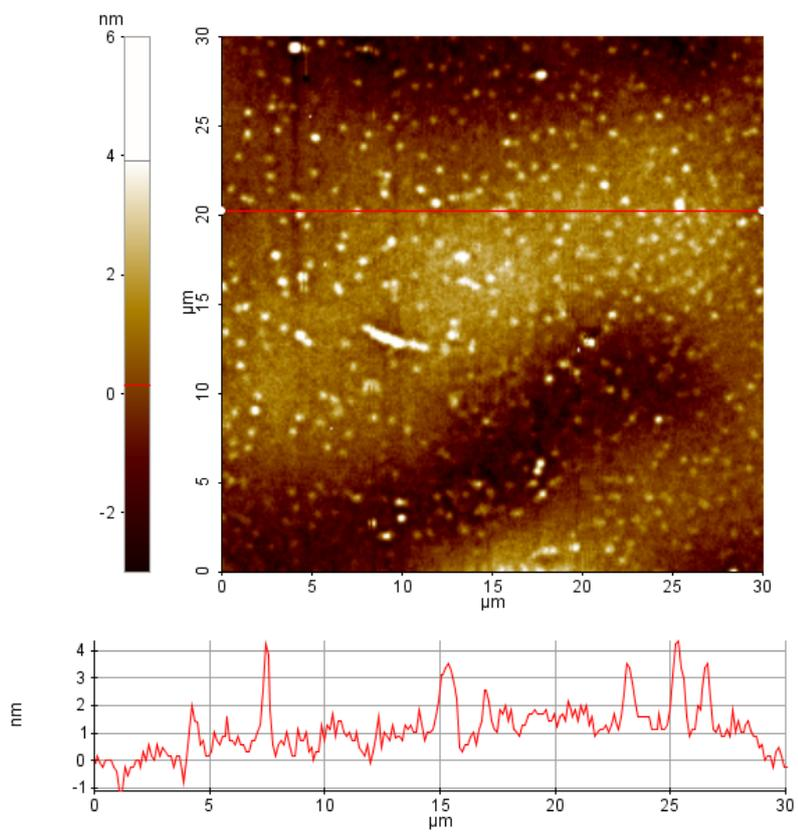
**Figure S3.** AFM image taken on a 30μm \*30 μm scale for DHI melanin thin film grown on glass. Below, the height profile caught from the red line on the image is reported.
