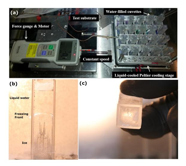
**Fig. S10.** (a) Photograph of the ice adhesion test apparatus showing 90% water-filled cuvettes that are inverted on test substrates and cooled at -15°C using a Peltier cooling stage for 2h to promote ice formation. (b) Image of ice being formed inside a cuvette and the solidification front. (c) Image of a cuvette after de-adhering from the substrate showing the state of the ice formed on the substrates and the smooth fracture interface.
