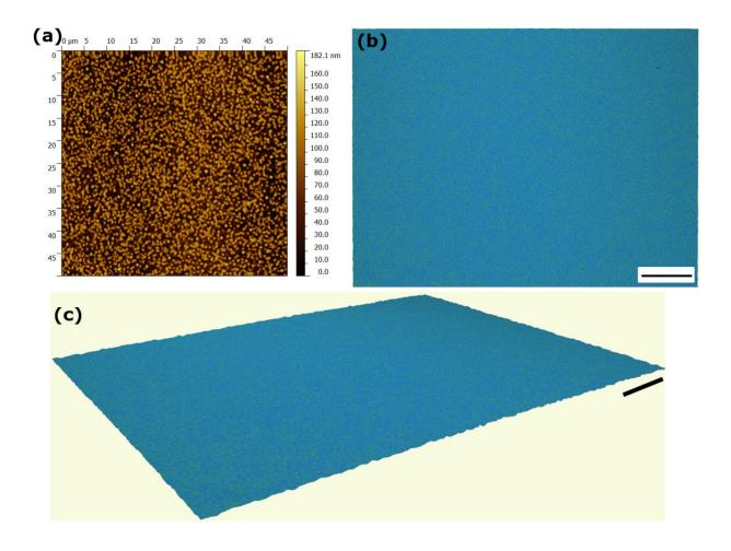
**Fig. S7.** (a) is AFM image, (b) and (c) are the top view and three dimensional optical profilometer images of the linker-free grafted bilayer pDVB/pPFDA with pPFDA thickness of ~ 10 nm deposited on the silicon substrate (BL (10 nm) on Si), respectively. AFM, and optical profilometer images show the presence of rough features in the BL (10 nm) on Si film with RMS roughness of  $R_q$ =28.3±3.8 nm. The scale bars in (b) and (c) are 20 μm.
