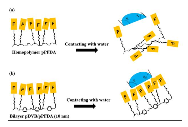
**Fig. S1.** Schematic of (a) homopolymer pPFDA and (b) bilayer pDVB/pPFDA with only 10 nm thick top layer pPFDA. The presence of highly cross-linked pDVB polymer layer underneath a very thin pPFDA fluoropolymer in (b) acts as a steric barrier resisting local surface reorganization, forcing the fluorinated groups to remain on the surface even under wet conditions.
