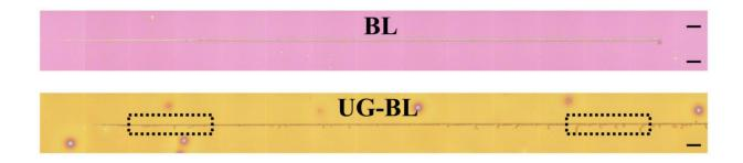
**Fig. S6.** Optical microscopy images obtained from the Nanovea mechanical tester after creation of a 2 mm long scratch on linker-free grafted bilayer pDVB/pPFDA (BL) (top) and ungrafted bilayer pDVB/pPFDA (UG-BL) (bottom). The UG-BL shows that the polymer delaminated frequently during the nanoscratch test while grafted polymers did not experience any sign of failure. The scale bar is  $50~\mu m$ .
