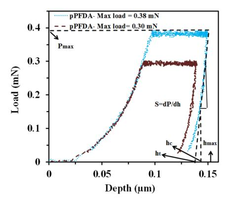
**Fig. S5.** Load/depth curves obtained from the nanoindentation measurements on the pPFDA film using 0.38 mN and 0.3 mN maximum load. The stiffness, S, is given by the slope of the unloading curve.
