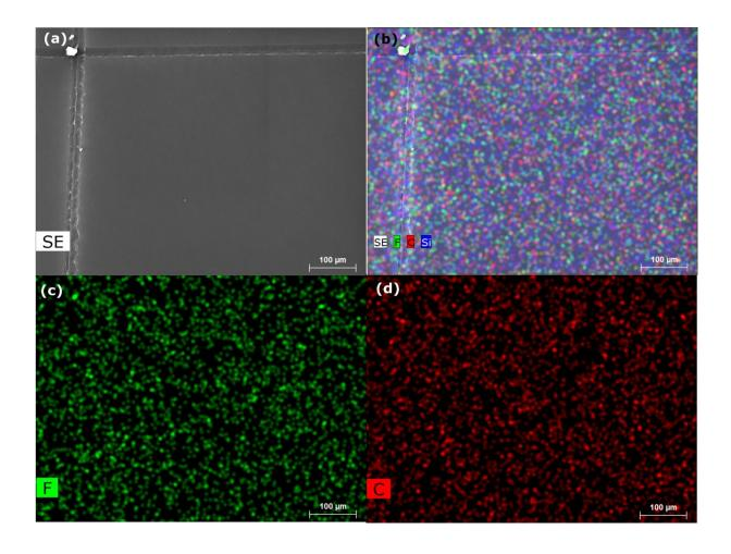
**Fig. S4.** (a) SEM-EDS micrograph and maps of distribution of elements on the linker-free grafted bilayer pDVB/pPFDA with pPFDA thickness of  $\sim 10$  nm deposited on the silicon substrate (BL (10 nm) on Si). The '+' mark is used as a fiducial reference to ensure that there is minimal drift in the images. The secondary electron (SE) image with Si, C, and F mapping in (b). The images in (c) and (d) reveal that carbon and fluorine species are uniformly distributed in the bilayer film.
