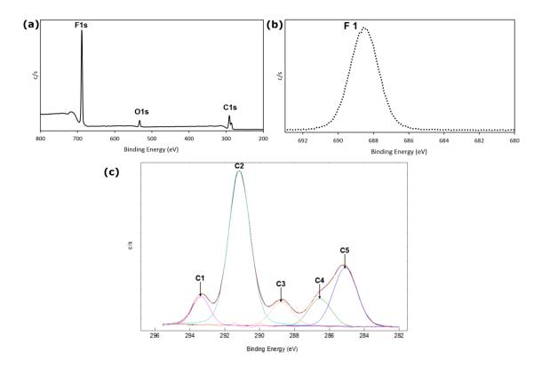
**Fig. S3.** (a) XPS survey spectra for detection of the atomic concentration of fluorine, oxygen, and carbon. (b) F1s high resolution XPS centered at 688.4 eV indicates the presence of fluorine groups. (c) High resolution C1s spectra with five resolved peaks (C1:  $-C*F_3$ , C2:  $-C*F_2$ , C3:-C\*=O, C4:  $-O-C*H_2-CH_2-$ , C5:  $-C-C*H_2-C-$ ).
