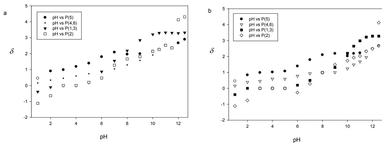
Supplemental Figure 3 Plot  $\delta$  in  $^{31}P$ -NMR vs. pH for a)  $H_n(IP)$  and  $(IP)H_n(Spm)$  systems
