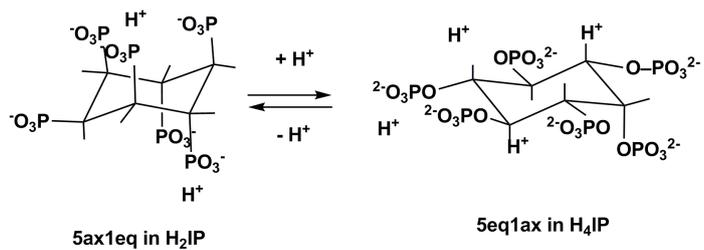
Supplemental Figure 5 Possible preferred conformations of 5ax1eq in H<sub>2</sub>IP and 5eq1ax in H<sub>4</sub>IP
