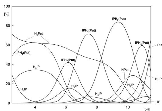
Supplemental Figure 2 Distribution diagram for IP/Put system. Percentage refers to total IP;  $c_{IP}=0.001M$ ,  $c_{Put}=0.001M$
