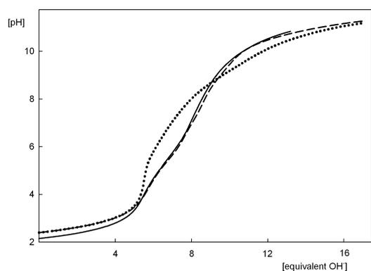
Supplemental Figure 1 Experimental and simulated titration curves for IP/Spm system.  $c_{IP}=c_{Spm}=0.001M$
