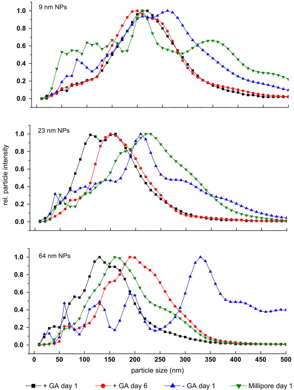
SI Fig. 4 Particle size distribution obtained via NTA (nanosight LM 20) in Hoagland medium without plants. Lines show difference in behavior of NPs in respect to NP-treatment, the legend is the same in all 3 sections
