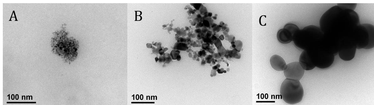
SI Fig 2. TEM images of  $\text{CeO}_2$  dispersed in Hoagland medium after 7 d. A) 9 nm  $\text{CeO}_2$ -NPs, B) 23 nm  $\text{CeO}_2$ -NPs, C) 64 nm  $\text{CeO}_2$ -NPs
