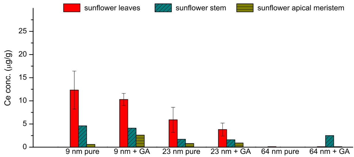
SI Fig.6 Ce-concentration in  $\mu\text{g/g}$  in the specific parts of sunflower shoots after treatment with the different NP-size-groups (x-axis).
