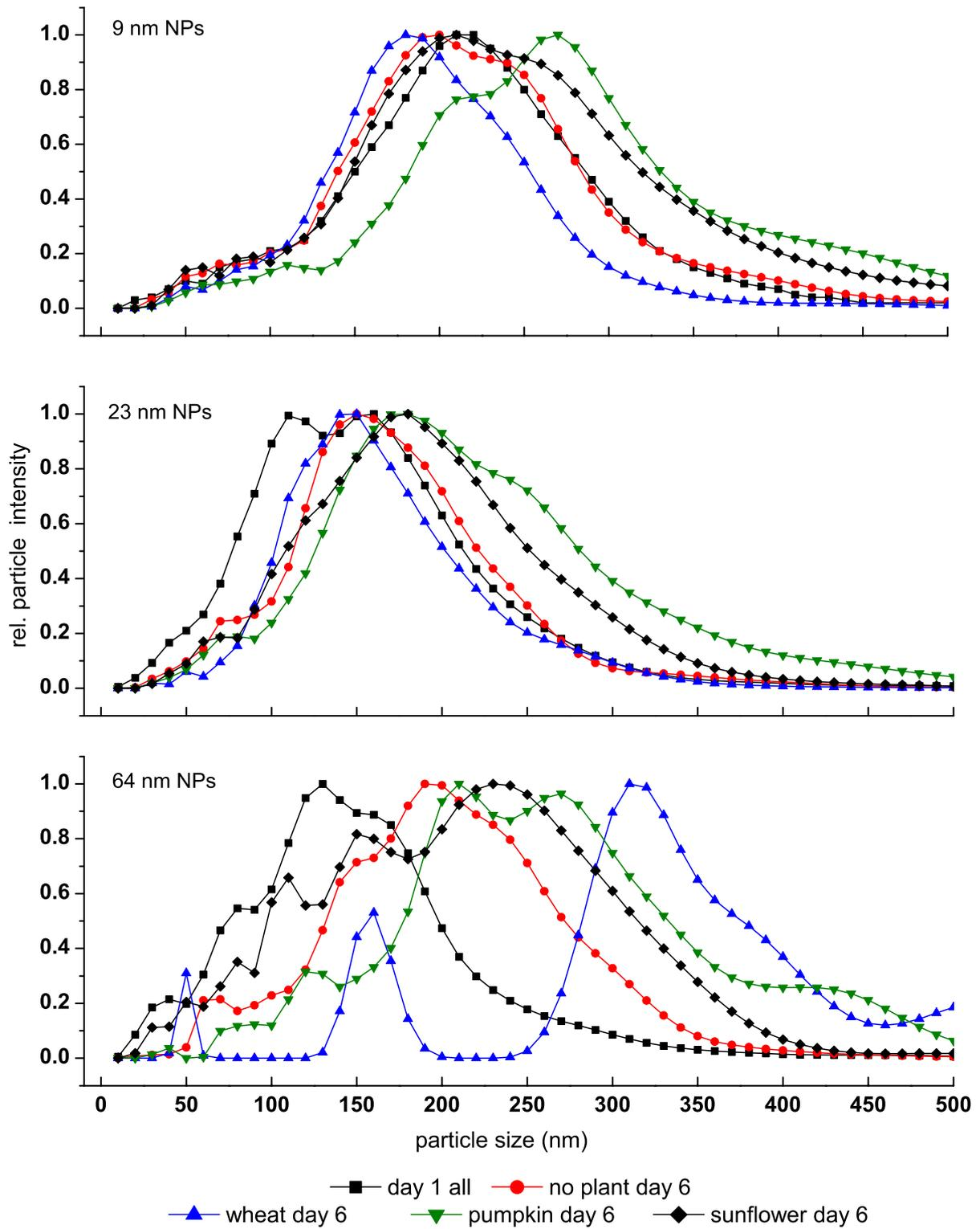
SI Fig. 5 Particle size distribution obtained via NTA (nanosight LM 20). Lines show difference in behavior of NPs in respect to plant species grown on the medium dispersion, the legend is the same in all 3 sections
