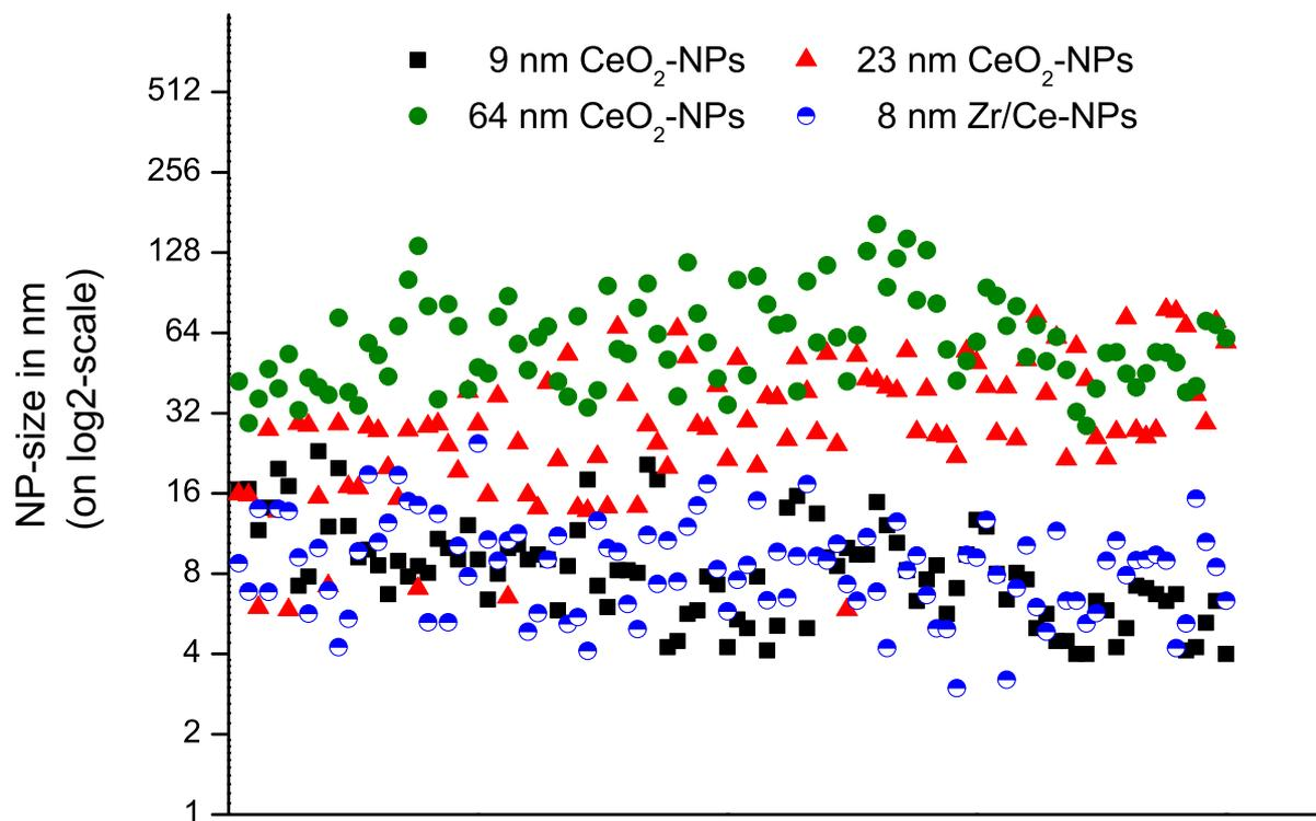
SI Fig. 3 Scatter plot of the size of 100 primary particles in each NP group, measured via TEM-image-recognition.
