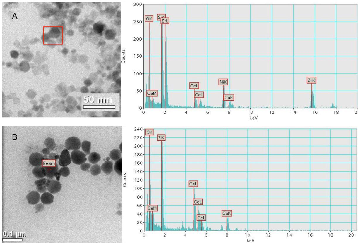
*SI Fig. 7 Control STEM-EDX images of Zr/Ce-NP. A) Image (left side) and EDX-Spectrum (right side) of Zr/CeO<sub>x</sub>-NPs centrifuged on grids right after dispersion in Millipore water. B) Images of particles found in control-leaves mixed with Ce<sub>2</sub>(SO<sub>4</sub>)<sub>3</sub>-powder before ashing, right side EDX-spectrum of indicated spot.*
