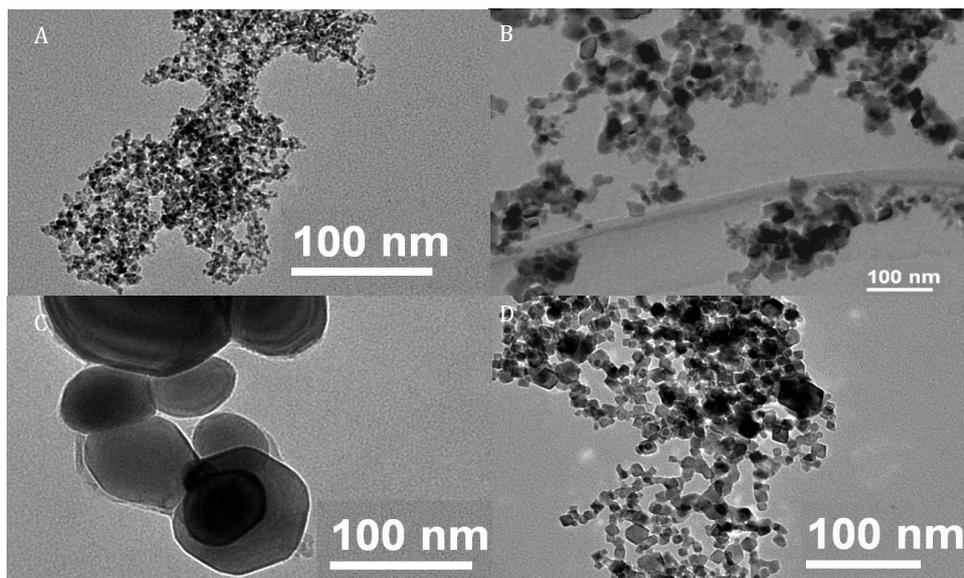
*SI Fig. 1 TEM images of  $\text{CeO}_2$  and  $\text{Zr/CeO}_x$  NPs in Millipore water; suspended with polyacrylamide. A) 9 nm  $\text{CeO}_2$  NPs, B) 23 nm  $\text{CeO}_2$  NPs, C) 64 nm  $\text{CeO}_2$  NPs, D) 9 nm  $\text{Zr/CeO}_x$  NPs*
