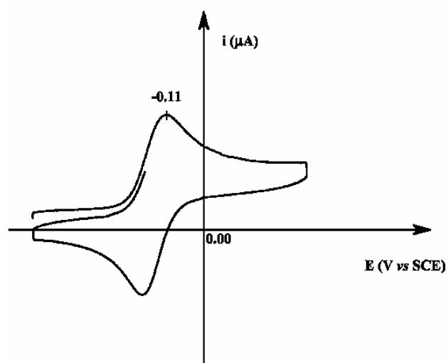
Cyclic voltammogram of DSeDAF **10**,  $\text{Bu}_4\text{NPF}_6$  (1 M),  $\text{CH}_2\text{Cl}_2$ , Pt working electrode, scanning rate 0.1 V/s
