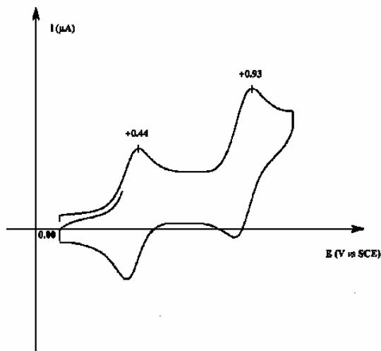
Cyclic voltammogram of azino-DSeDAF **12**,  $\text{Bu}_4\text{NPF}_6$  (1 M), MeCN, Pt working electrode,
