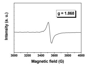
ESR spectrum measured at 298 K of the  $NaP_5W_{30}/PEI$  sample after 10 min of UV irradiation by a 500 W high pressure Hg lamp.
