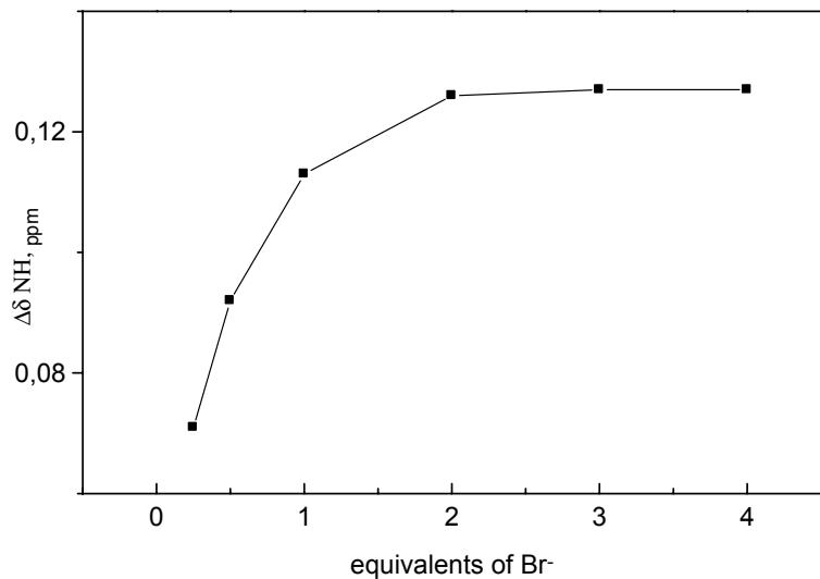
Variation of  $\delta_{\text{(NH)}}$  of calixarene derivative **4** in presence of  $\text{Bu}_4\text{NBr}$ , ( $\text{CDCl}_3$ ).
