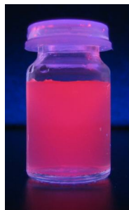
Figure S7. \text{Eu}_2(\text{bdc})_3(\text{H}_2\text{O})_4 nanoparticles in PVP re-dispersed in water after irradiation at \lambda = 312 nm.
