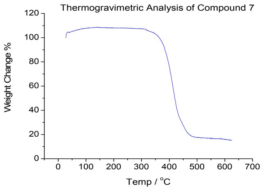
TG curve of compound **7** (typical of all samples) showing decomposition of the sample occurs above 300 °C.
