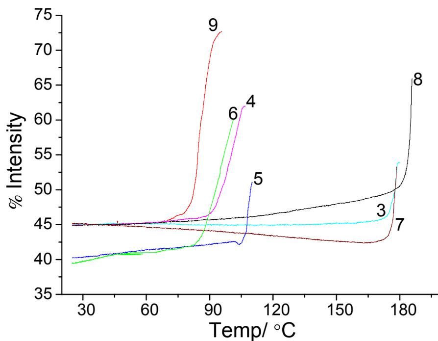
HSM heating curves as a function of intensity; all samples were heated at a rate of 5°C/min.
