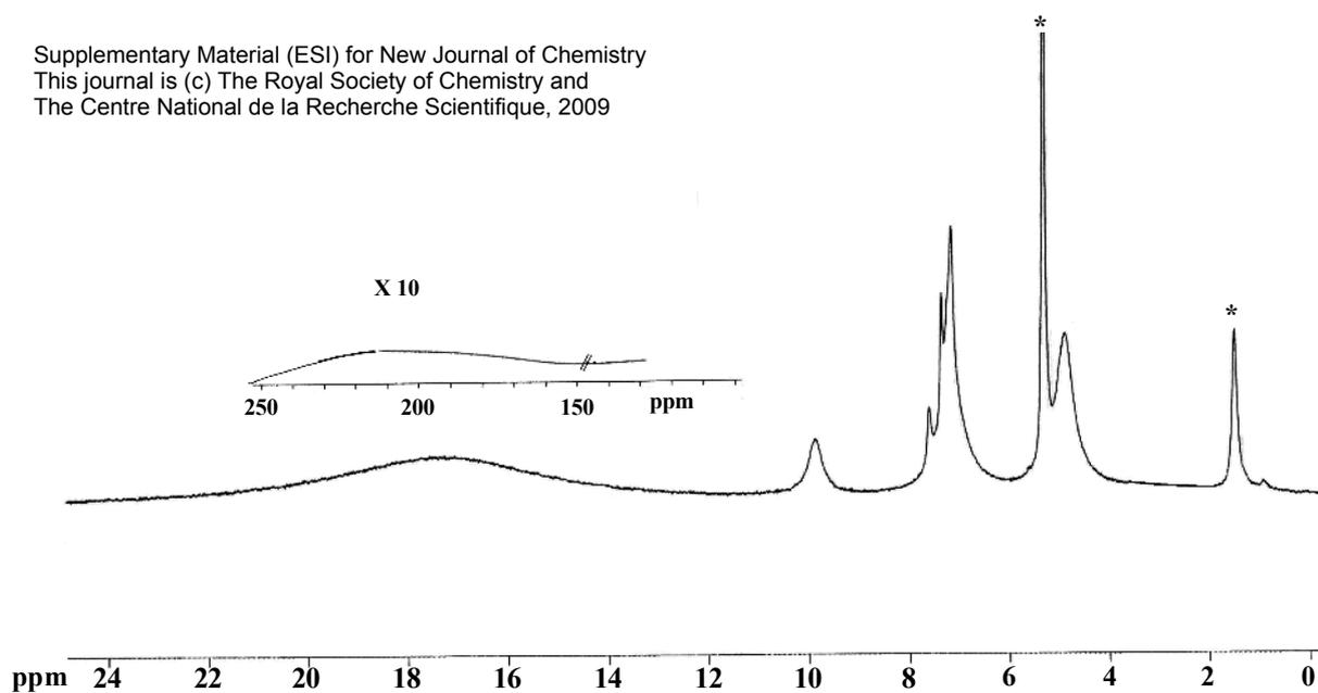
**Fig. S2** Proton NMR spectra of  $[\text{Fe}_2(m\text{-xba})_2(\mu\text{-OCH}_3)_2]\cdot\text{CH}_2\text{Cl}_2$  (**1**) in  $\text{CD}_2\text{Cl}_2$ . Asterisks show peaks due to the solvent.
